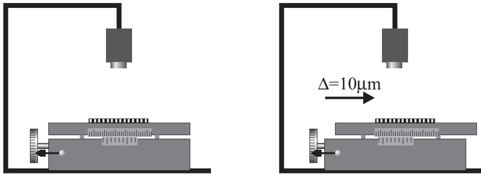
Figure 4.31: To test the accuracy, the IC was mounted on a precise xy\varphi -stage, which can be shifted with an accuracy of 1\ \mu\text{m} and can be rotated with an accuracy of 0.7' ( 0.011667^\circ ).
