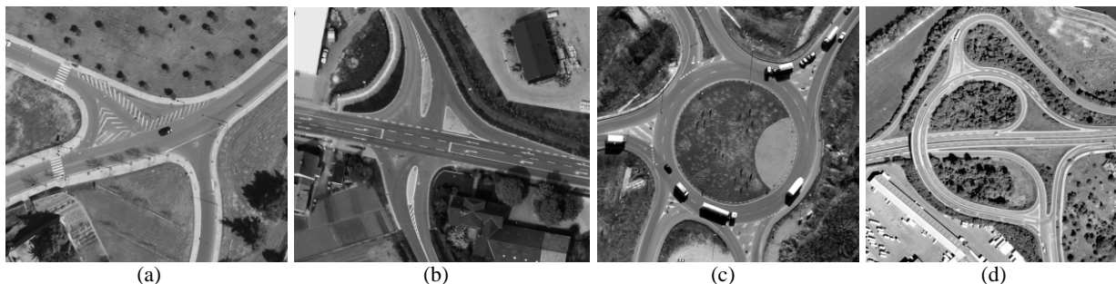
Figure 3-1: Junction classes. (a) Simple junction. (b) Complex junction. (c) Roundabout as a subclass of complex junction. (d) Motorway junction.
