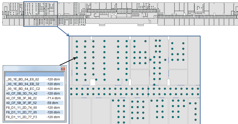
Figure 255: Grid points for the sixth floor (top) and example fingerprint measured at a single grid point (bottom).
