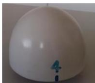
Abb. 4.5: Trimble Bullet III Antenne
