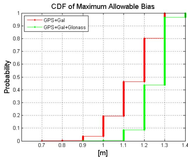
Figure 9-10: CDF of Maximum Allowable Bias (on All Satellites)
