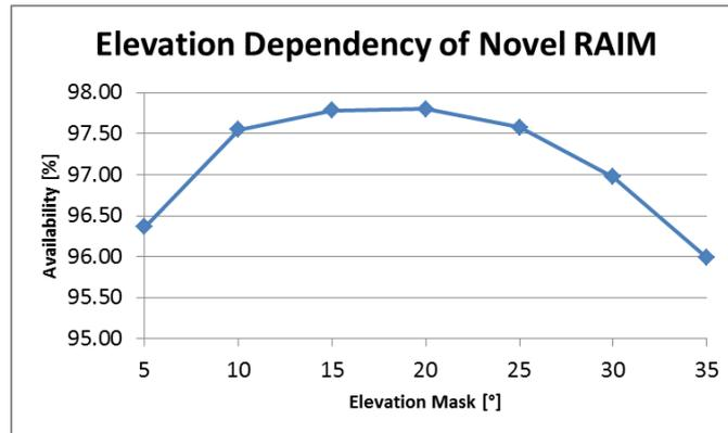
Figure 8-19: Availability of Integrity as function of Elevation Mask
