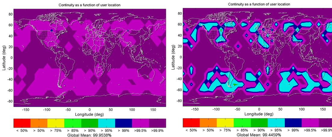
Figure 8-15: Continuity (Novel RAIM) as function of user location (left: 15 min CTI; right: 3 h CTI), GPS+Gal
