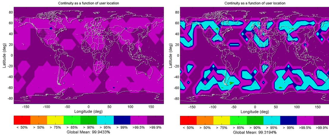
Figure 8-13: Continuity (LSR RAIM) as function of user location (left: 15 min CTI; right: 3 h CTI), GPS+Gal
