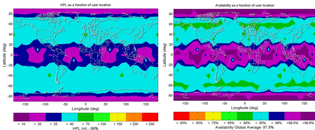
Figure 8-7: HPL (left) and Availability (right) as function of user location, nominal biases considered, GPS only (masking angle 20°)
