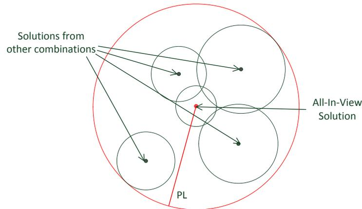
Figure 5-14: The concept of Protection Level computation for the Solution Separation approach
