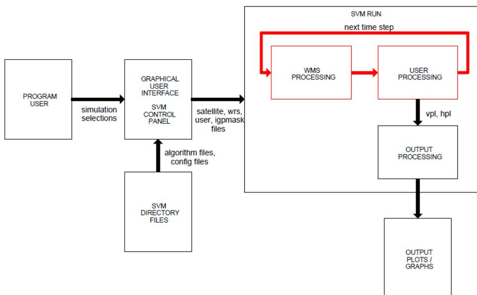
Figure A-1: Service Volume Model (SVM) Analysis Block Diagram (Top Level View)
