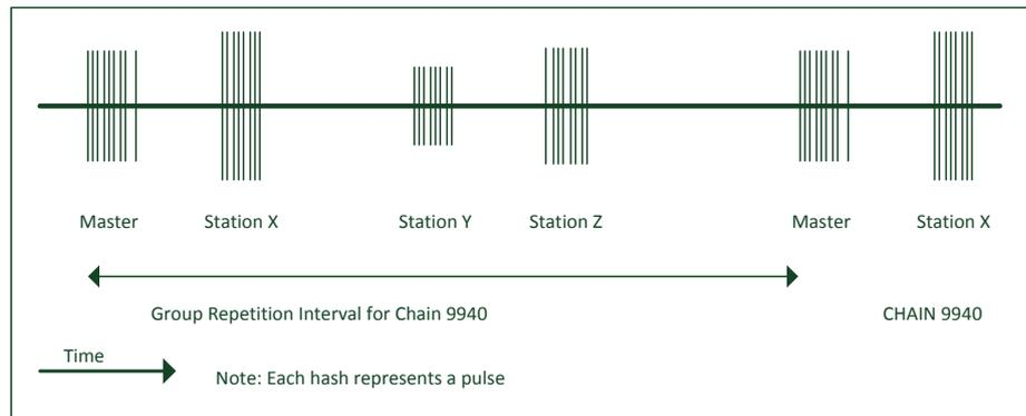
Figure 2-2: LORAN Chain Signals [Sherman 2003]
