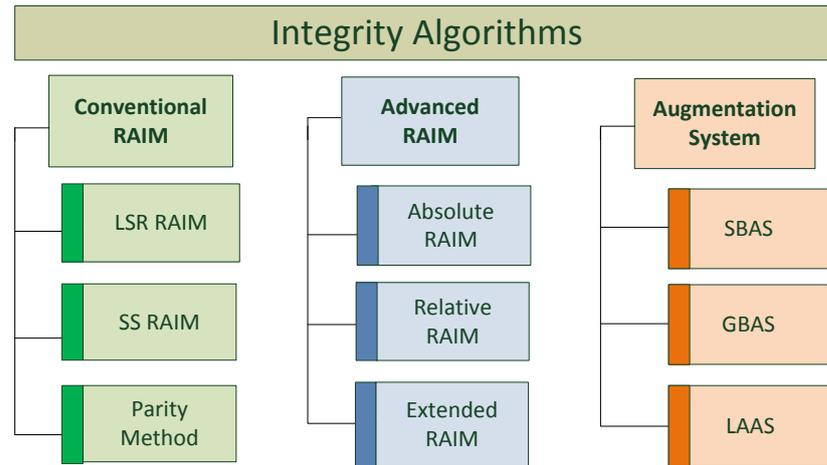
Figure 5-1: Overview of Integrity Algorithms
