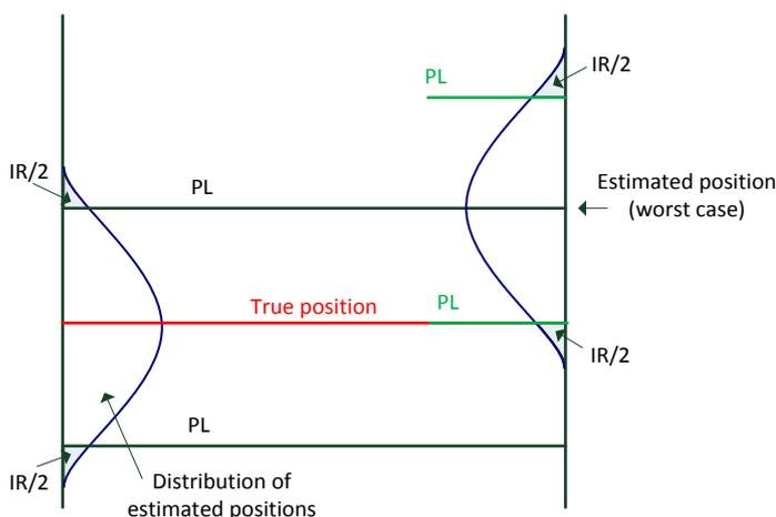
Figure 3-3: Relationship of Protection Level centered around True and Estimated Position
