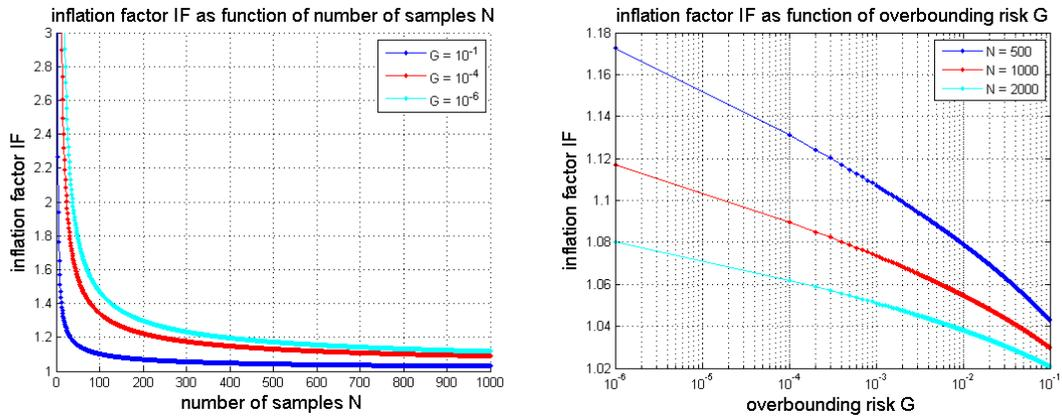
Figure 9-6: Inflation factors as function of number of samples  $N$  (left) and of overbounding risk  $G$  (right)
