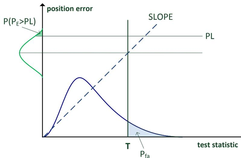
Figure 5-3: Illustration of Protection Level Calculation based on Mapping of T
