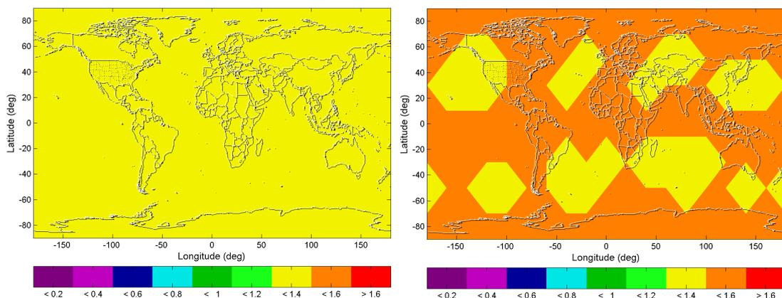
Figure 9-11: Maximum Allowable Bias on All Satellites for dual (left) and triple (right) constellation scenario (maximum values per user location)
