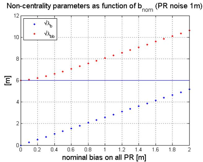
Figure 5-7: Non-centrality parameters  $\lambda(b)$  and  $\lambda(bb)$  as function of  $b_{nom}$
