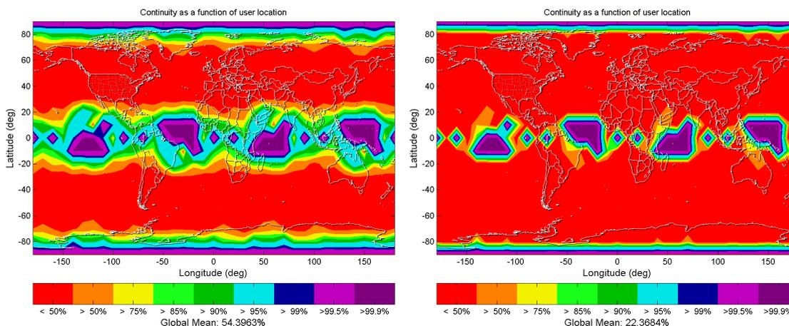
Figure 8-12: Continuity (LSR RAIM) as function of user location (left: 15 min CTI; right: 3 h CTI), GPS only
