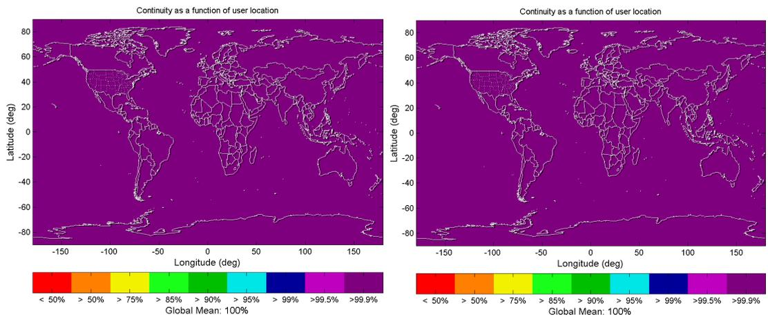
Figure 8-17: Continuity (MHSS RAIM) as function of user location (left: 15 min CTI; right: 3 h CTI), GPS+Gal
