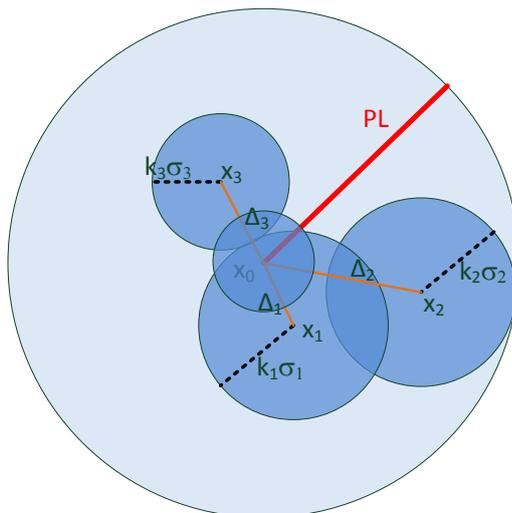
Figure 5-15: Protection Level Calculation using MHSS Algorithm
