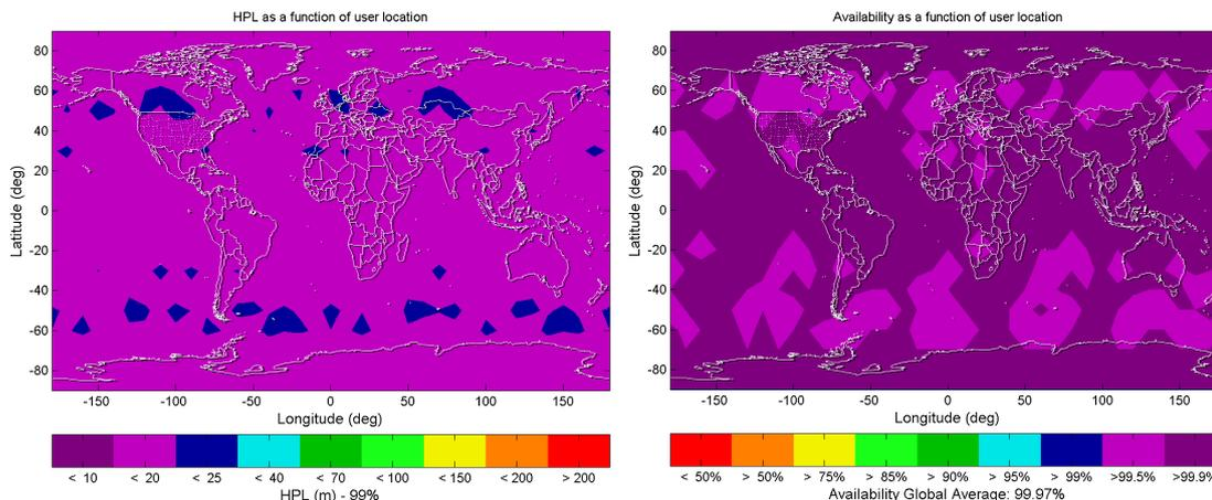
Figure 8-8: HPL (left) and Availability (right) as function of user location, nominal biases considered, GPS+Gal (masking angle 20°)
