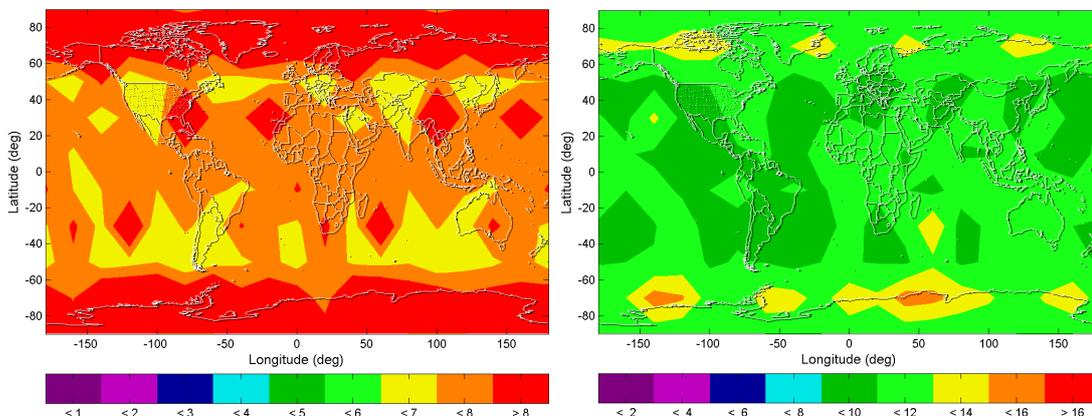
Figure 9-8: Maximum Allowable Bias on the Critical Satellite for dual (left) and triple (right) constellation scenarios (maximum values per user location)
