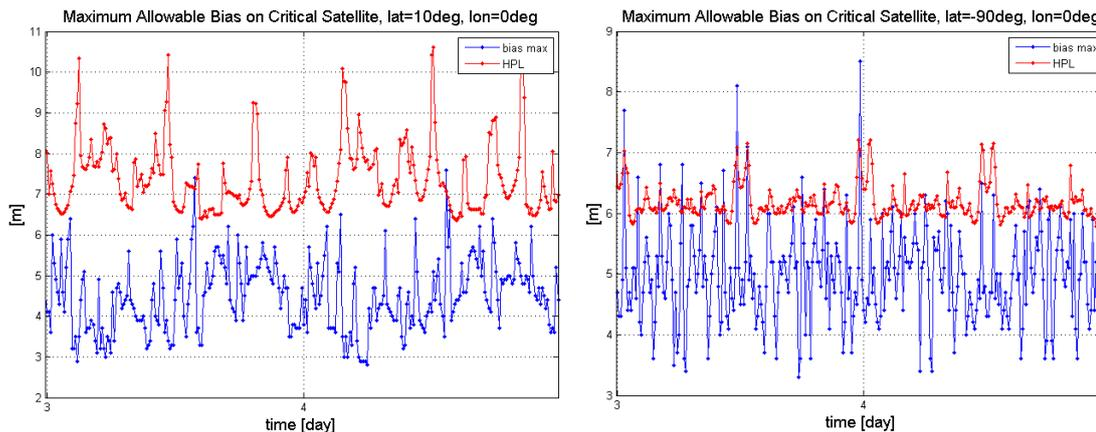
Figure 9-9: Maximum Allowable Bias versus its HPL over Time (GPS+GAL). Left: polar region; right: equatorial region
