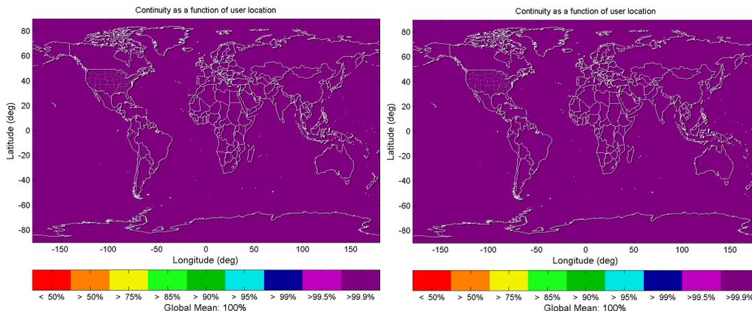
Figure 8-18: Continuity (MHSS RAIM) as function of user location (left: 15 min CTI; right: 3 h CTI), GPS+Gal+GLO
