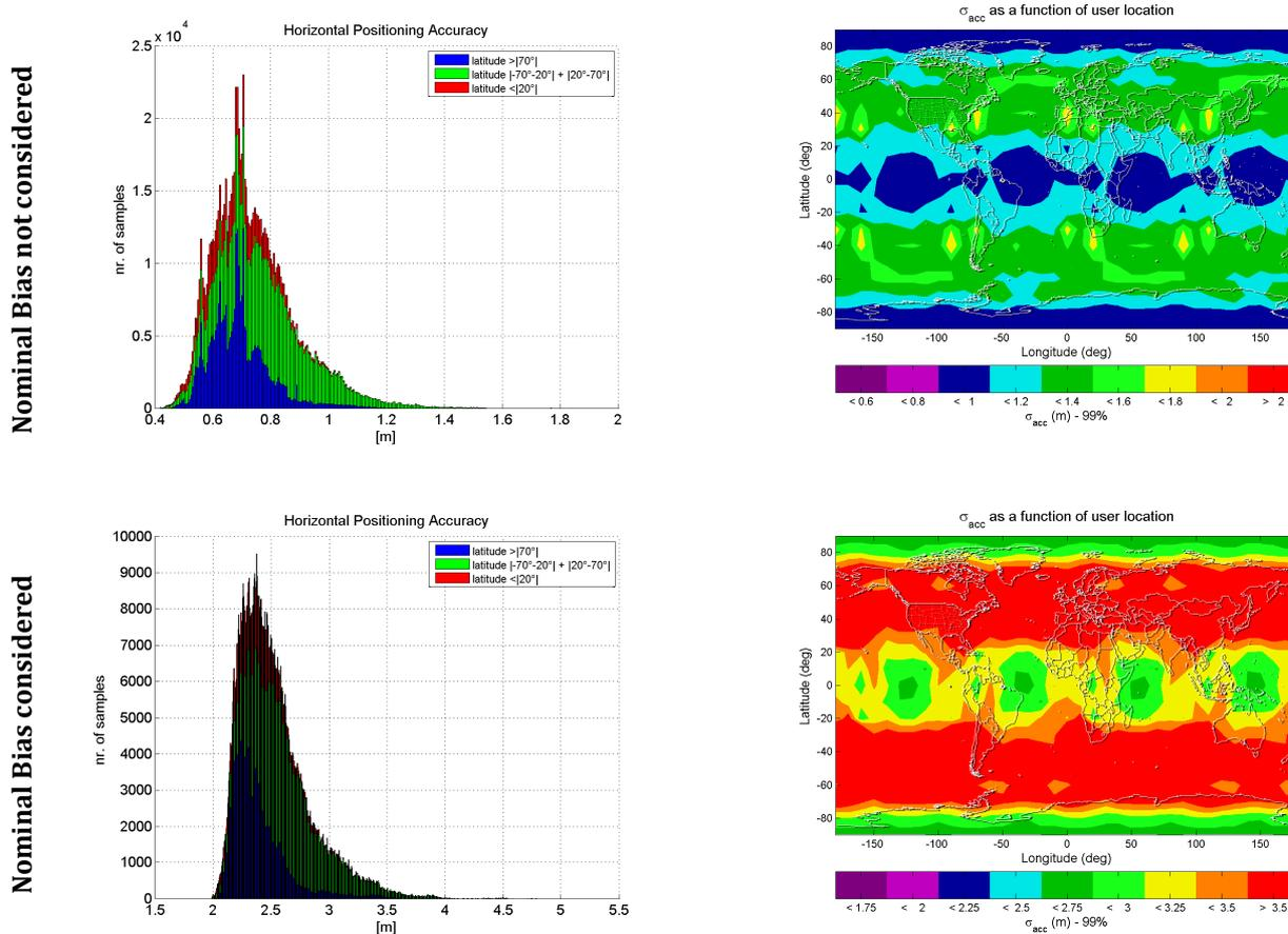
Figure 8-1: Horizontal Position Accuracy (left: PDF over all grid points and epochs; right: Position Accuracy as function of User Location) – GPS only
