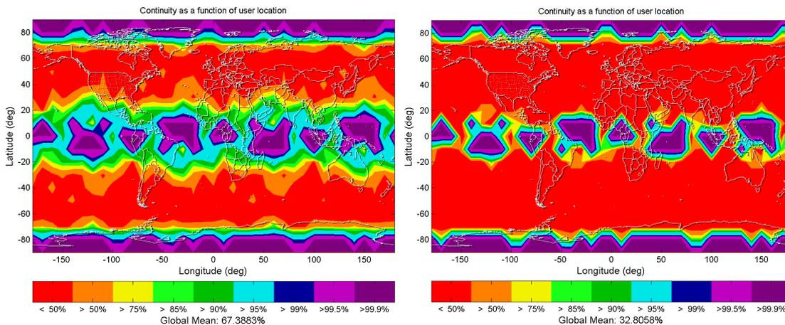
Figure 8-14: Continuity (Novel RAIM) as function of user location (left: 15 min CTI; right: 3 h CTI), GPS only
