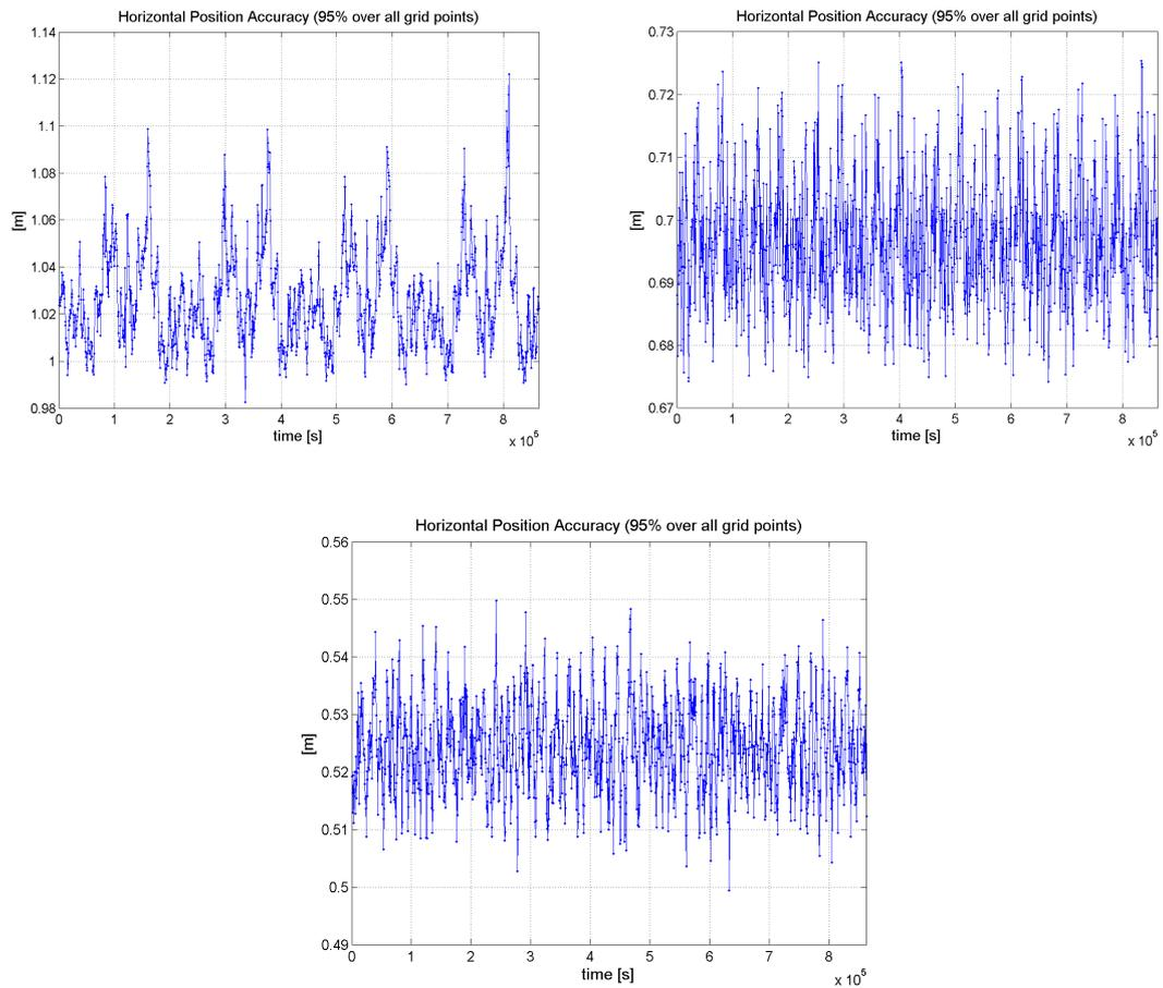
Figure 8-4: Horizontal Position Accuracy shown as 95-percentile over all grid points as function of time (nominal biases neglected); top left: GPS only, top right: GPS+Gal, bottom: GPS+Gal+GLO
