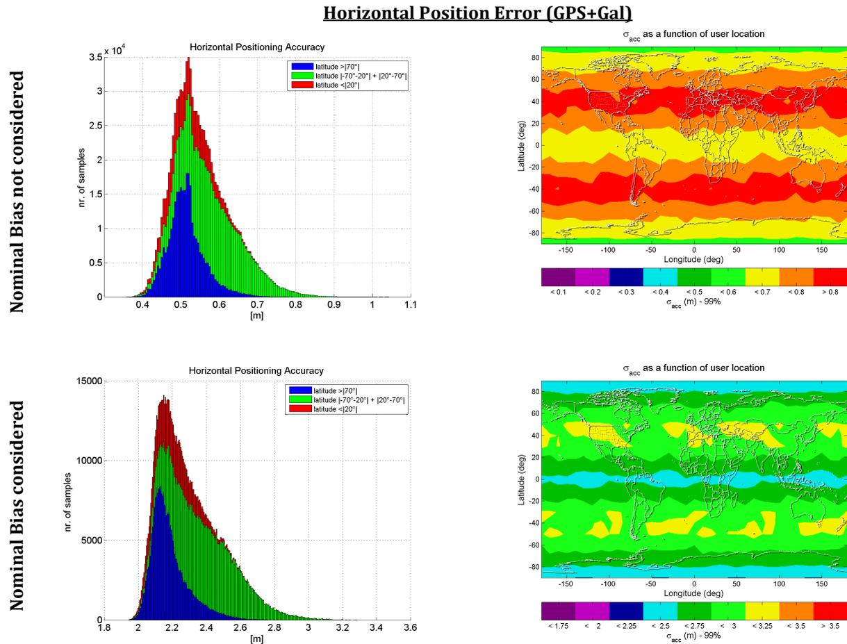
Figure 8-2: Horizontal Position Accuracy (left: PDF over all grid points and epochs; right: Position Accuracy as function of User Location) – GPS+Gal
