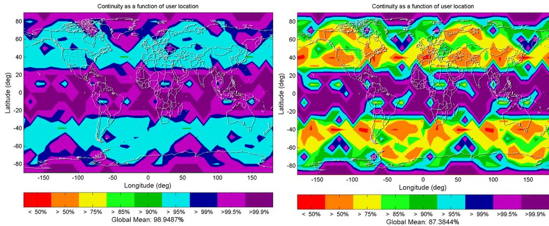
Figure 8-16: Continuity (MHSS RAIM) as function of user location (left: 15 min CTI; right: 3 h CTI), GPS only
