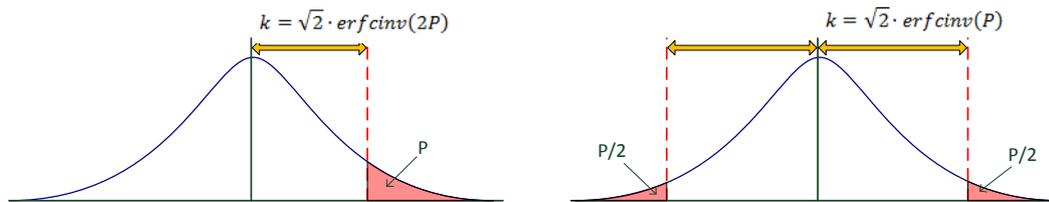
Figure 3-4: k-factor based on one (left) or two (right) tails contributing to probability P
