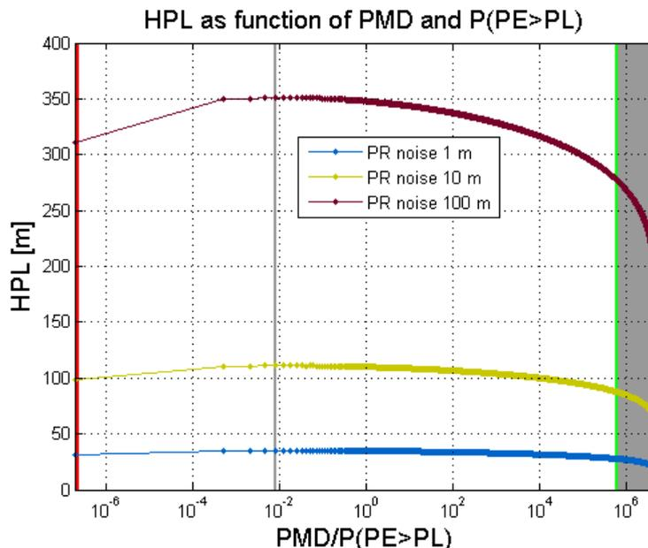
Figure 5-5: HPL as Function of PMD and P(PE>PL)
