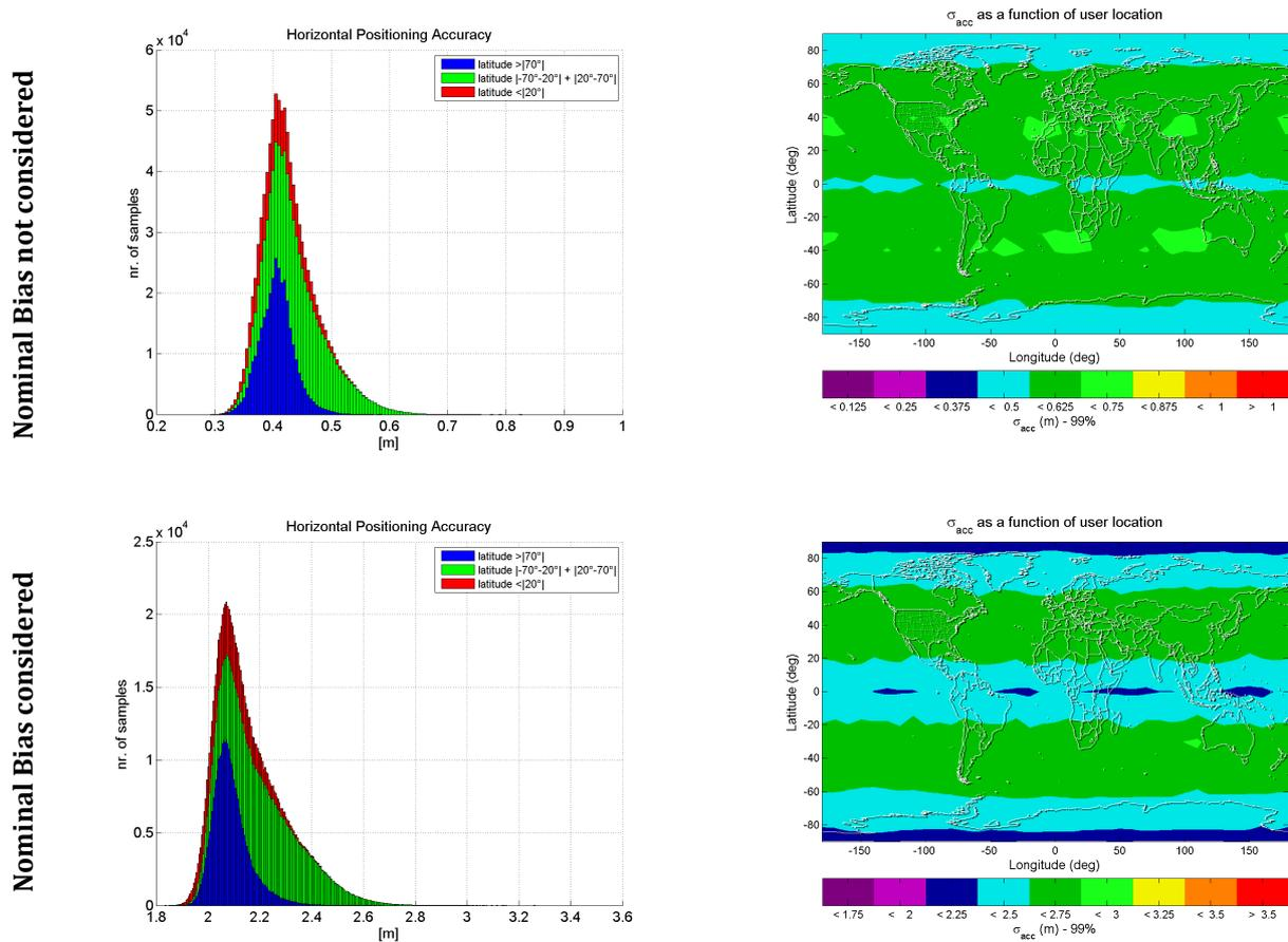
Figure 8-3: Horizontal Position Accuracy (left: PDF over all grid points and epochs; right: Position Accuracy as function of User Location) – GPS+Gal+GLO
