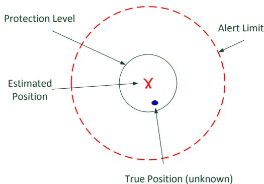
Figure 3-2: Definition of a Protection Level
