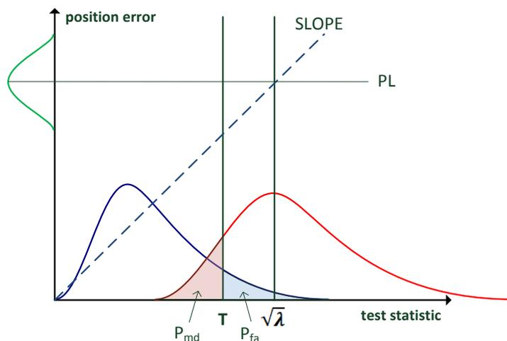
Figure 5-4: Illustration of Protection Level Calculation based on Mapping of Pbias
