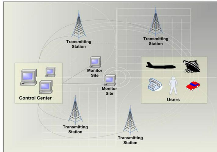
Figure 2-3: eLORAN System Concept [International Loran Association 2007]
