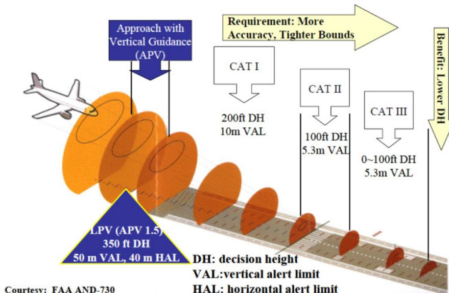
Figure 4-4: Alert Limit Evolution for Aircraft Precision Approaches [ICAO 2006b], [Pullen et al 2002]
