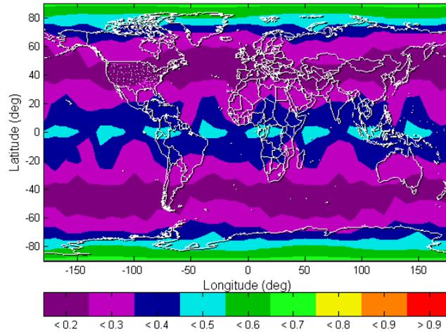
Figure 5-11: Availability of FD pre-condition based on GPS only (masking angle 20°)
