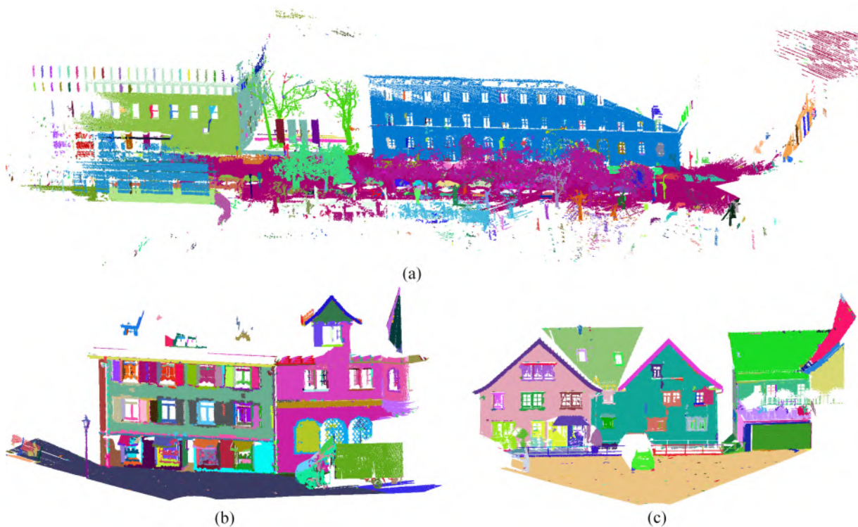
Figure 8.34: Illustration of segmentation results using GGBC. (a) Segmentation result of the TUM scene (Arcisstrasse), (b) segmentation results of the Town Square scene (Sample 4), and (c) segmentation results of the St. Gallen scene (Sample 5).
