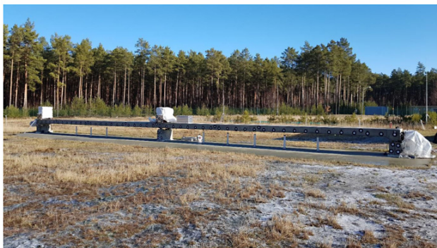
Figure 33: A scheme of the BAM synthetic bridge, which was measured by the MEMS accelerometers, the geophone, the laser tracker Leica AT960-LR and the IATS Leica MS50.
