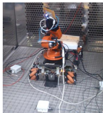
Figure 2. A calibration experiment using a KUKA youBot inside the climate chamber at the Institute of Thermodynamics, Leibniz University Hannover.
