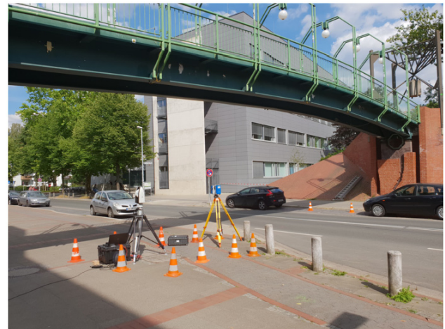
Figure 12: A scheme of the Mensa footbridge, which was measured by the MEMS and high-end (reference) accelerometers, the laser tracker Leica AT960-LR and the terrestrial laser scanner Z+F IMAGER 5016.
