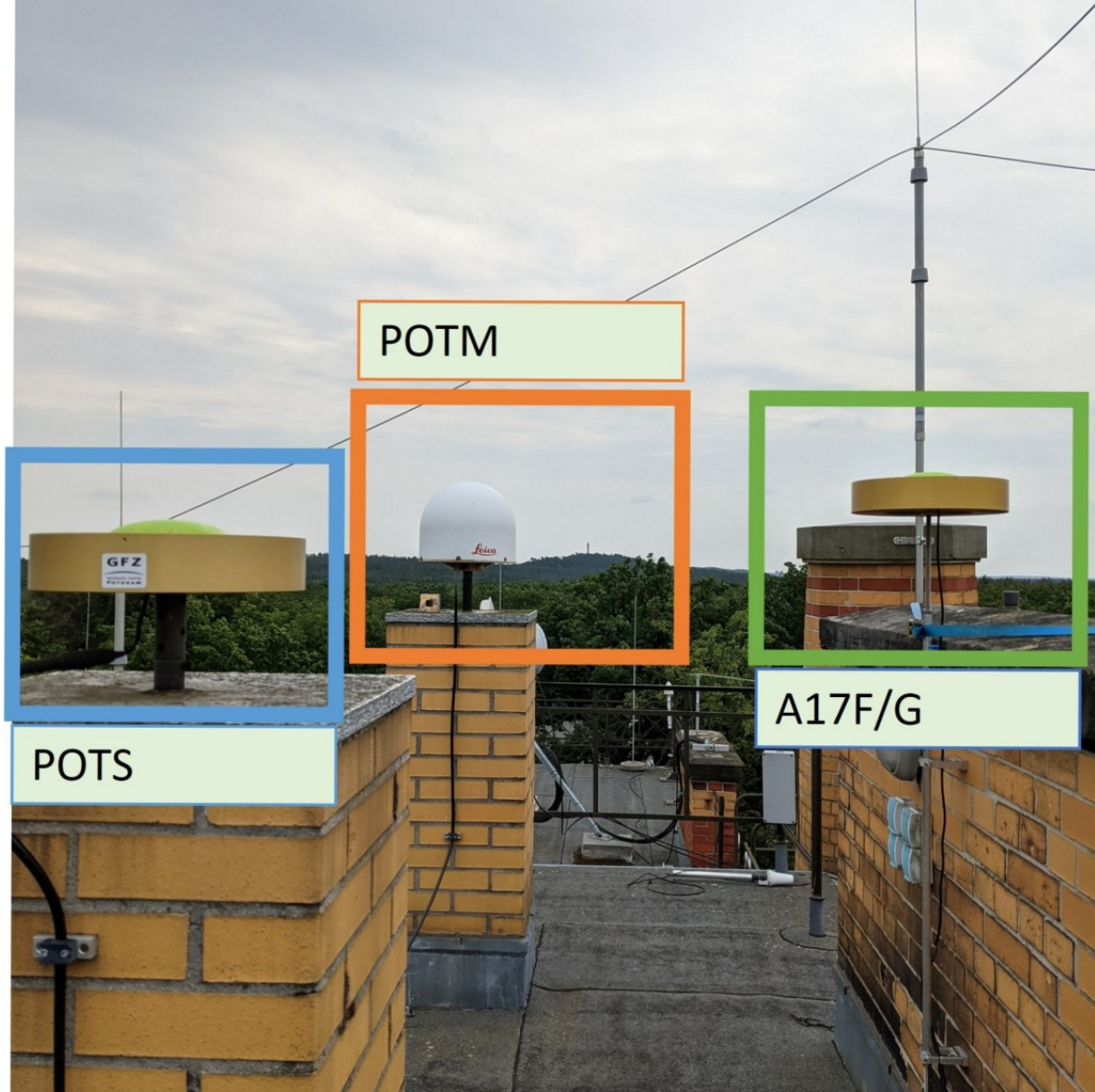
Figure 4.4: The GNSS co-location experiment set-up on the rooftop of A17 building (Telegrafenberg, Potsdam Germany). Two permanent GNSS stations, namely POTS and POTM, were placed on a similar level and continuously operated. The experimental station A17F/G was attached to a vertical steering pole that allows the mitigation of height shift when changing the antenna during the experiment. The picture was taken from Kitpracha et al. (submitted)).
