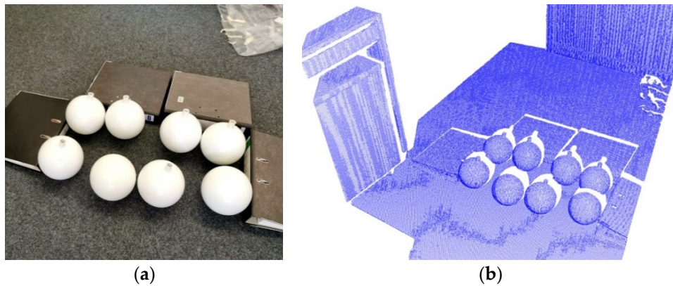
Figure 5.27: The multiple-sphere scanning test: (a) The placement of multiple spheres; (b) Preprocessed point cloud (voxel size in downsampling: 3 \times 3 \times 3 \text{ mm}^3 ) (Yang et al. , 2021).
