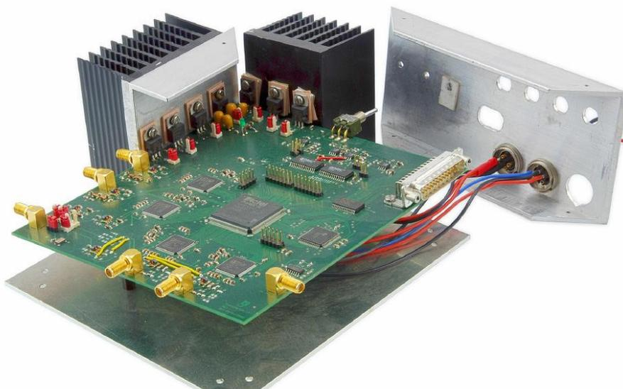
**Figure 5-31:** A typical 4 channel FPGA based phasemeter developed at AEI Hannover.
