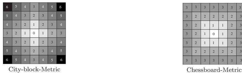
Figure A.1.: Distances from the central pixel using different metrics in  $\mathbb{Z}^2$
