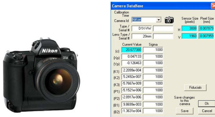
Figure 5.1: A Nikon D1X professional digital camera with its calibration results
