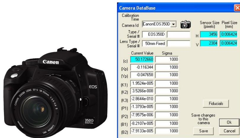
Figure 7.4: The Canon EOS 350D camera with its calibration parameters result
