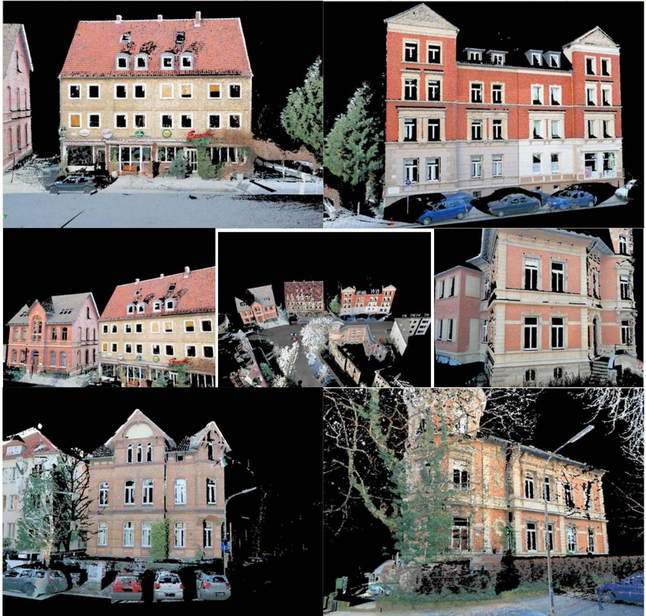
Figure 5.15: Some snapshots from the colored point cloud of the T-section
