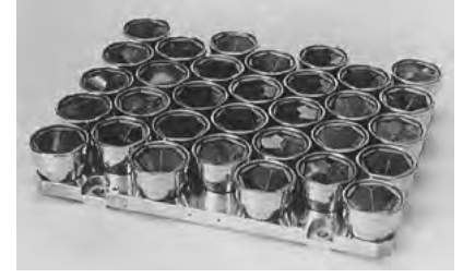
Fig. 7.10: LRA used onboard SVN 35 and 36 (Degnan and Pavlis, 1994).
