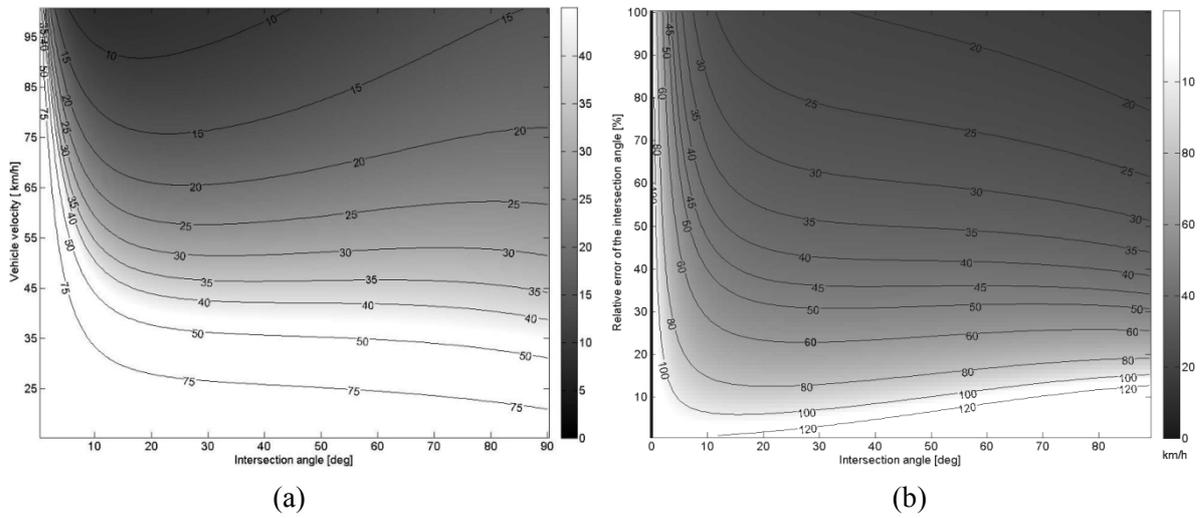
Figure 37: Accuracy of the intersection angle obtained based on the joint estimation of velocity and heading, (a) standard deviation  $\sigma_{\theta_v}$  as a function of target velocity  $v$  and the intersection angle  $\theta_v$ ,  $\sigma_{\theta_v}$  is given in degree; (b) Relative error of the intersection angle  $\sigma_{\theta_v}/\theta_v$
