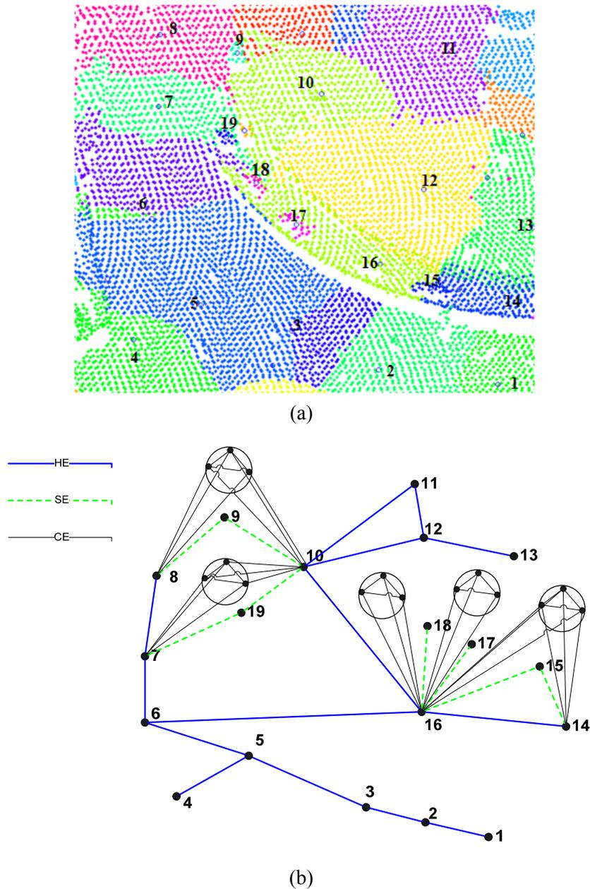
Figure 18: **RAG** for point segments (a): Numbered point segments for the section (black dotted box) of Figure 16(b), (b): the corresponding non-planar RAG with multi child-nodes (within each black circle, for point segments 9, 15, 17, 18, 19, respectively), each point segment is represented as a node in the graph
