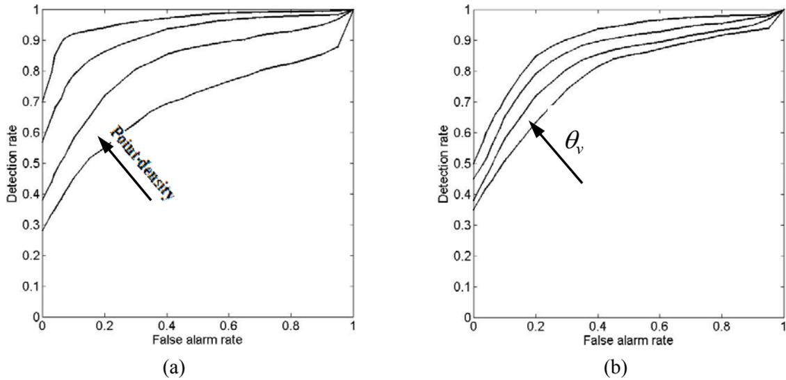
Figure 52: ROC curves of the motion detector using the Lie group metric (a) for point densities of (from innermost to outermost) – 2 points/m<sup>2</sup>, 4 points/m<sup>2</sup>, 7 points/m<sup>2</sup>, and 10 points/m<sup>2</sup>, (b) for different relative moving directions of vehicles (from outermost to innermost:  $\theta_v = 0^\circ$ ,  $\theta_v = 30^\circ$ ,  $\theta_v = 90^\circ$ , and  $\theta_v = 60^\circ$ ). Here, the point density is fixed at 4 points/m<sup>2</sup>
