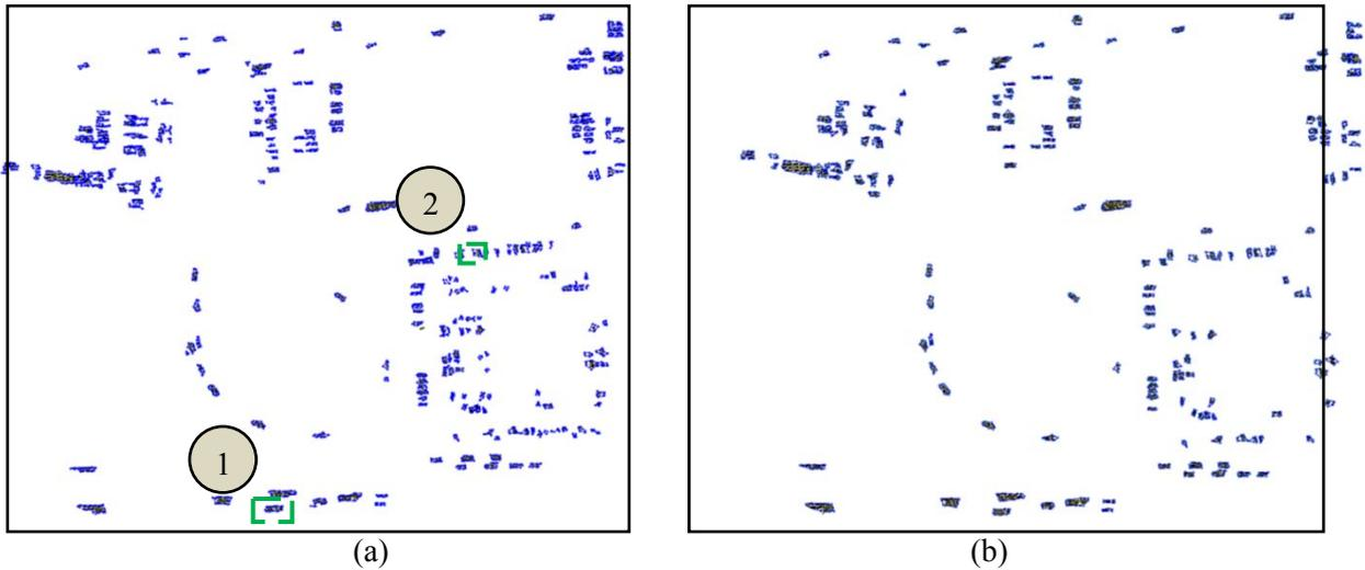
Figure 29: Example for vehicle shape parameterization: (a) boundary tracing, (b) boundary regularization
