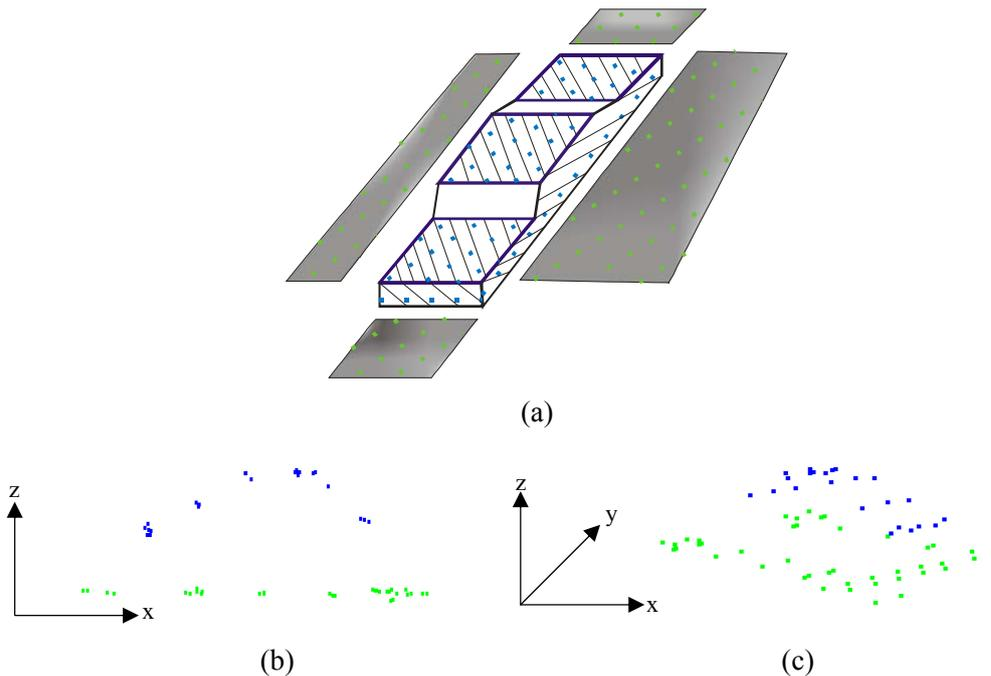
Figure 3: Vehicle model and point cloud (green: ground, blue: vehicle), a) schematic 3D vehicle model. Measured point cloud in b) side view and c) oblique view
