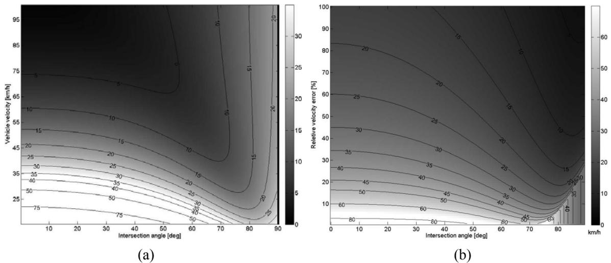
Figure 38: Accuracy of vehicle velocities obtained based on the joint estimation of velocity and heading, (a) standard deviation  $\sigma_v$  as a function of target velocity  $v$  and the intersection angle  $\theta_v$ ,  $\sigma_v$  is given in km/h; (b) Relative velocity error  $\sigma_v/v$
