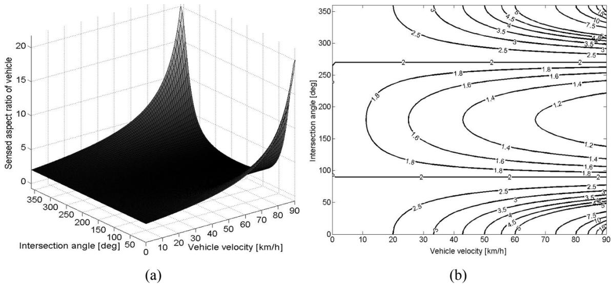
Figure 24: Stretching effect of a moving object in ALS data, (a) as function of  $\theta_v$  and  $v$  while  $v_L=100$  km/h, (b) contour plot of (a)
