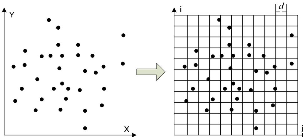
Figure 10: Schema of geo-tiling for LiDAR points indexing
