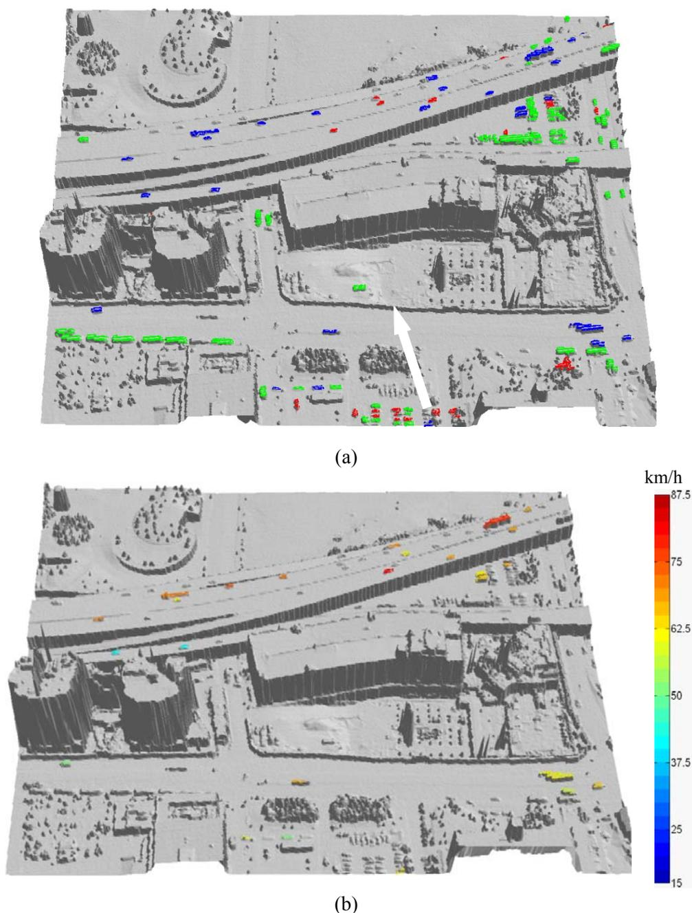
Figure 44: Vehicle motion analysis results for dataset Toronto II: (a) motion state classification, (b) velocity estimation
