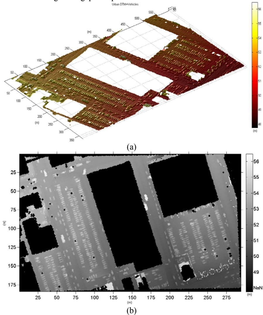
Figure 11: Filled height raster of ground points with surface fitting, black areas indicate object points masked out, (a) perspective-view; (b) top-view
