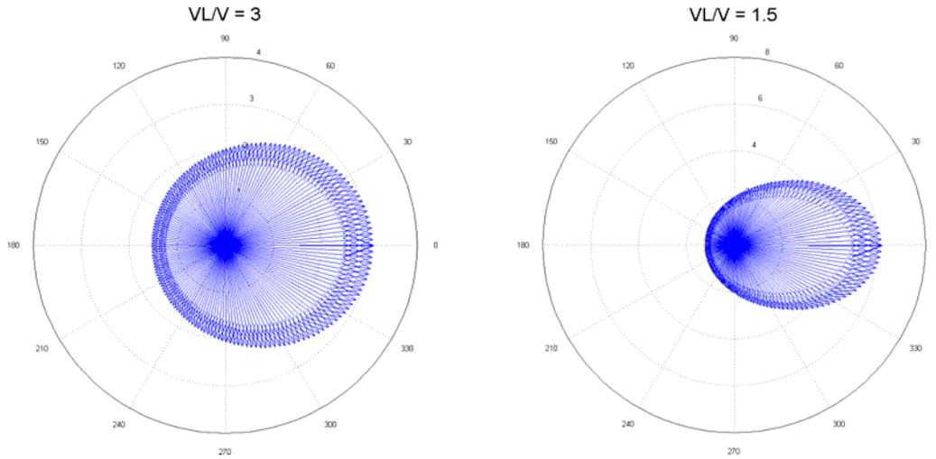
Figure 25: Visualization of the sensed aspect ratio  $Ar_s$  in polar coordinate system as the function of the intersection angle  $\theta_v$ , as the velocity ratio of sensor flight to moving target  $v_L/v$  changes from 3 to 1.5
