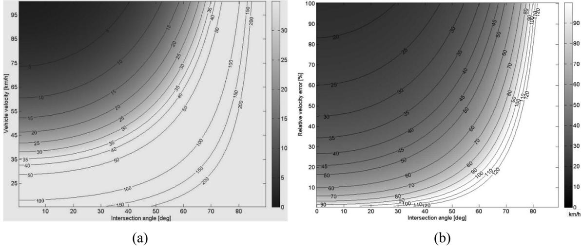
Figure 34: Accuracy of vehicle velocities estimated from the along-track stretching effect, (a) standard deviation  $\sigma_v^a$  as a function of target velocity  $v$  and the intersection angle  $\theta_v$ ,  $\sigma_v^a$  is given in km/h; (b) Relative velocity error  $\sigma_v^a/v$
