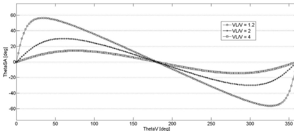
Figure 27: Shearing effect of a moving object in ALS data as function of  $\theta_v$ , when the velocity ratio of sensor flight to moving target  $v_l/v$  is fixed. Lines of different styles depict different velocity ratios used for simulation
