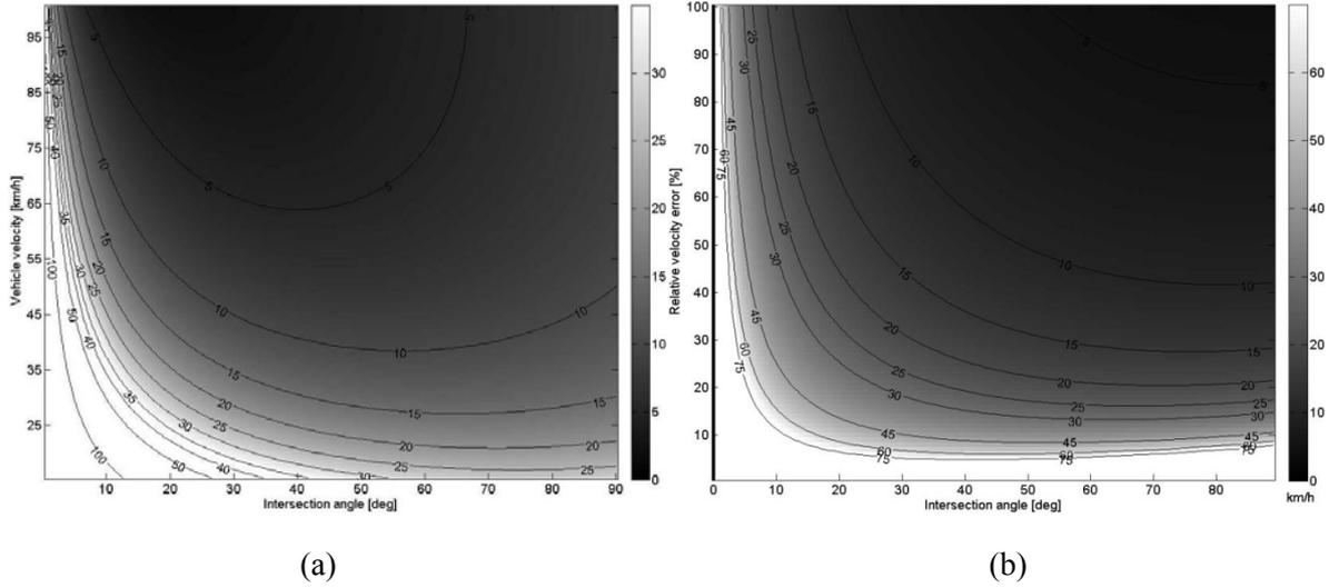
Figure 33: Accuracy of vehicle velocities estimated from the across-track shearing effect, (a) standard deviation  $\sigma_v^c$  as a function of target velocity  $v$  and the intersection angle  $\theta_v$ ,  $\sigma_v^c$  is given in km/h. (b) Relative velocity error  $\sigma_v^c/v$
