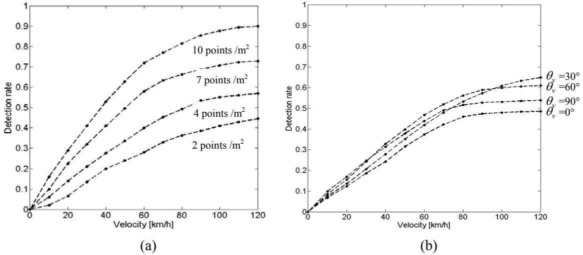
Figure 53: Numerical Detection Characterization: detection probabilities for given fixed false alarm rate ( $10e-2$ ): (a) results calculated for varying vehicle sizes (i.e. point density), (b) results calculated for varying relative moving directions; Here, the point density is fixed at 4 points/m<sup>2</sup>
