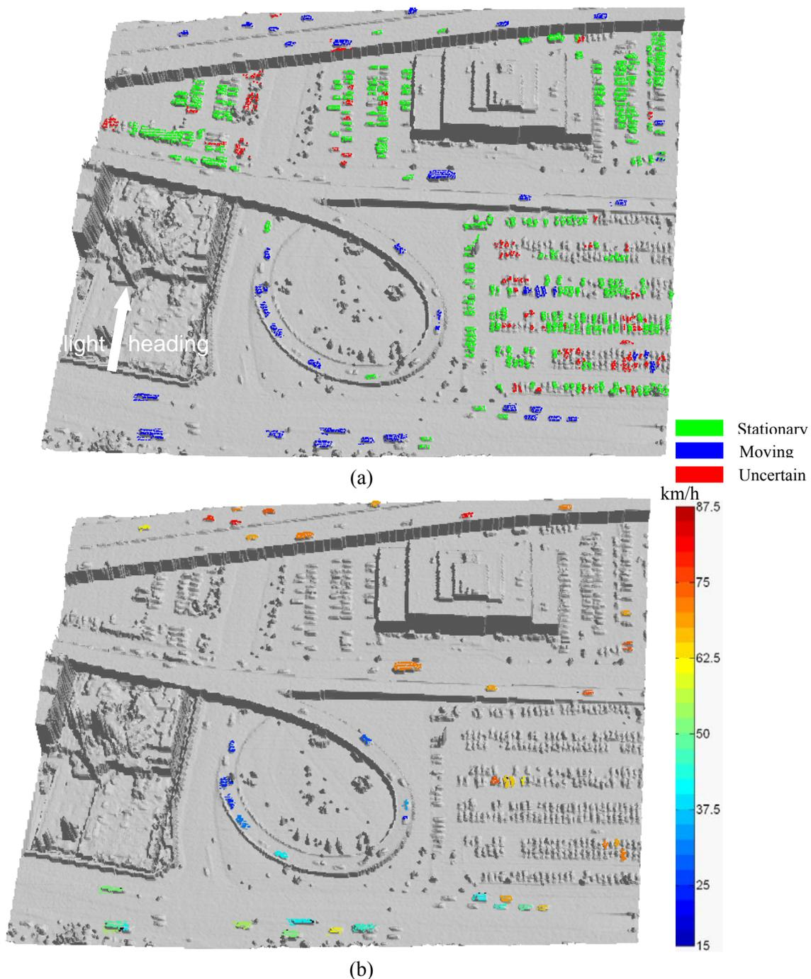
Figure 43: Vehicle motion analysis results for dataset Toronto I: (a) motion state classification, (b) velocity estimation
