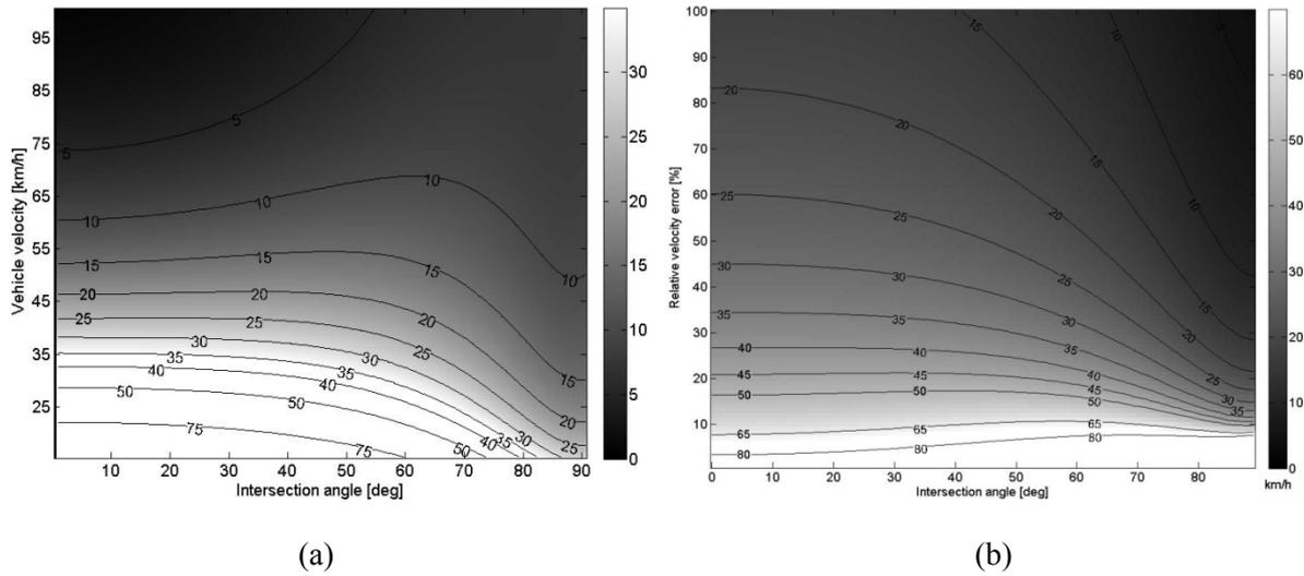
Figure 36: Accuracy of vehicle velocities estimated based on combining the two velocity components, (a) standard deviation  $\sigma_v^{a+c}$  as a function of target velocity  $v$  and the intersection angle  $\theta_v$ ,  $\sigma_v^{a+c}$  is given in km/h; (b) Relative velocity error  $\sigma_v^{a+c}/v$
