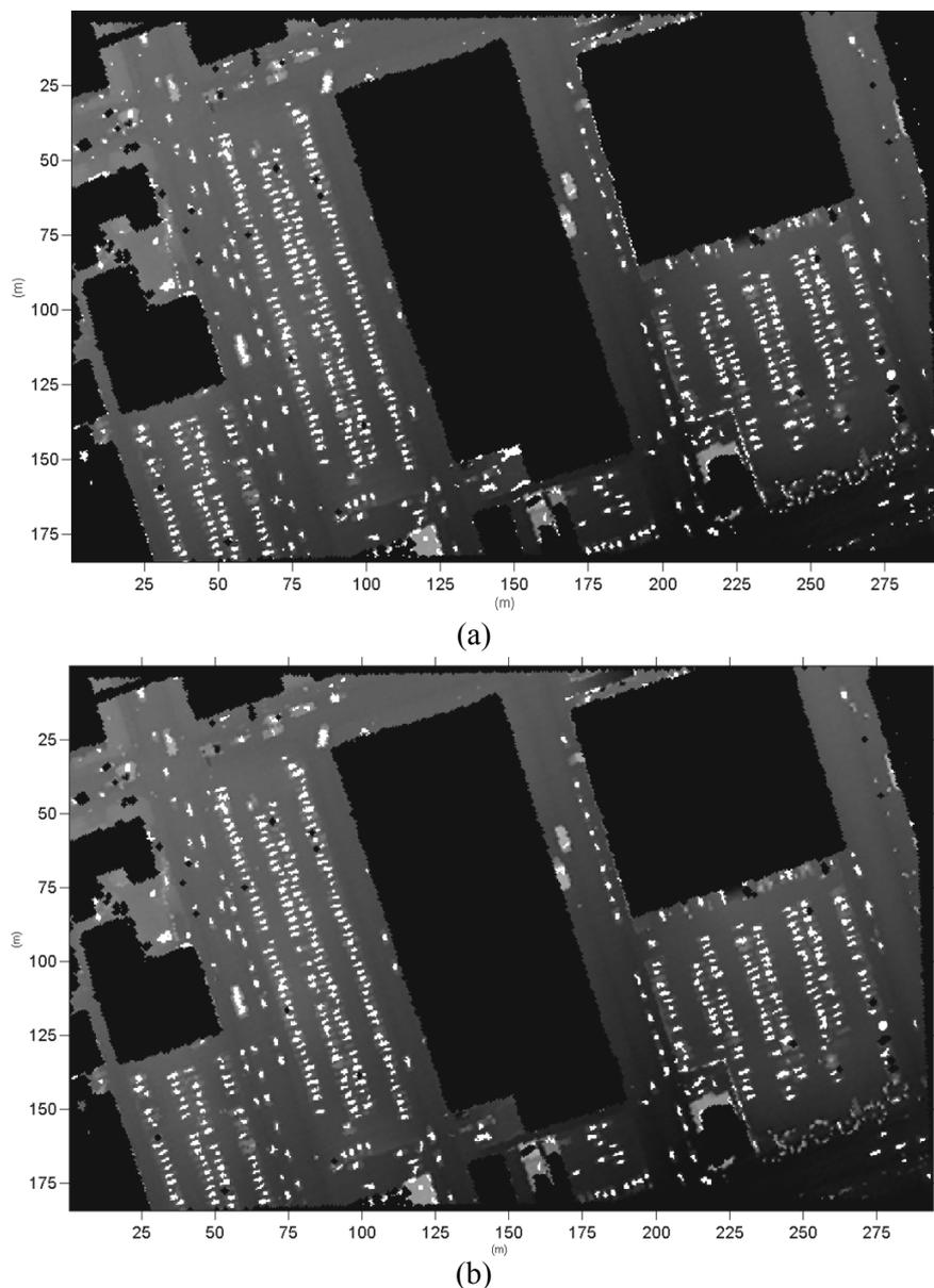
Figure 12: Detected vehicle-tops (white blobs) superimposed on Figure 11, (a) before refinement, (b) after refinement
