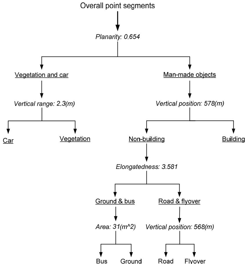
Figure 20: Classification tree for assigning the urban categories to segments in [Figure 19](#), the threshold values were learned by training data extracted from the same dataset
