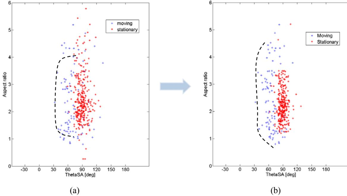
Figure 32: Transformation of a feature space of vehicle shapes of two motion states using PGA: (a) original feature space, (b) feature space after PGA. The shearing angle  $\theta_{SA}$  for moving vehicle class is normalized into the acute angle range ( $\leq 90^\circ$ ) for simplicity. Black dotted lines indicate the possible lines of separation
