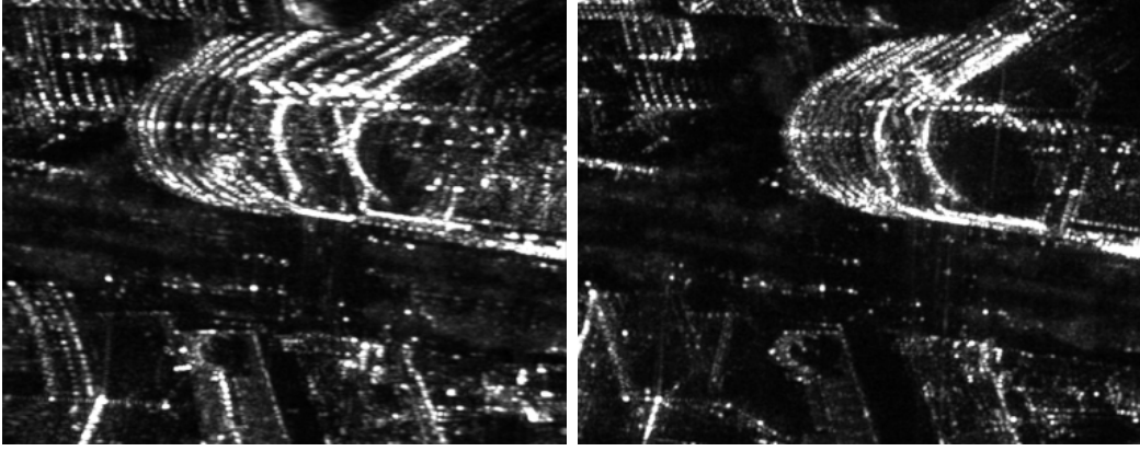
Fig. 11. Spotlight TerraSAR-X data showing the range shift corresponding to elevated scatterers for different look angles of the SAR. The facade of the imaged building is characterized by metal structures and glass. Left: Building shape in SAR image for look angle of approx. 27^\circ . Right: Building shape in SAR image for look angle of approx. 38^\circ . The range coordinate corresponding to elevated scatterers changes with the look angle of the SAR (Goel and Adam, 2010).
