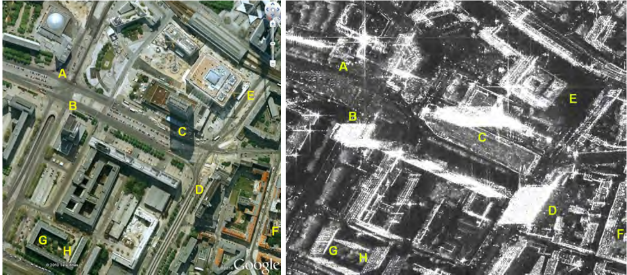
Fig. 7. Optical image and TerraSAR-X temporal average image of the Alexanderplatz in Berlin, Germany. Left: Bird's eye view (screenshot from Google Earth™ viewer; ©AeroWest, 2010). Large buildings marked by letters A – D. Right: SAR temporal average image derived by averaging 21 spotlight VHR TerraSAR-X images captured in VV-polarization. Angle of incidence: 47^\circ . Letters E, F, G, and H mark examples for shadow, foreshortening at gable roofs, double bounce at building walls, and point patterns corresponding to building facades, respectively. Azimuth: bottom-up; Range: from left to right.
