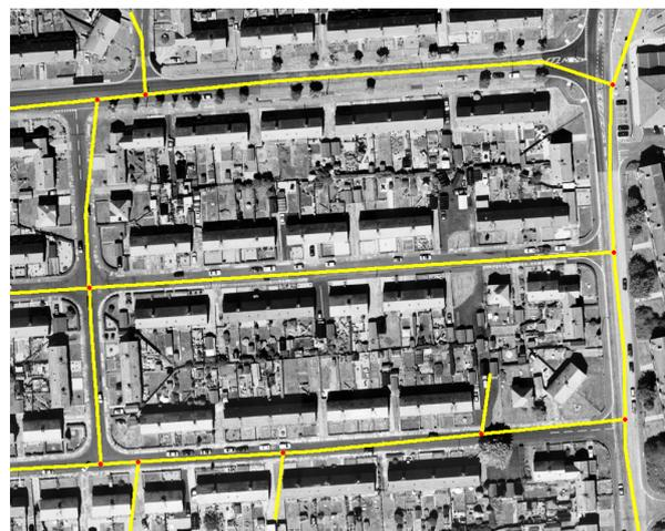
Figure 5.12. Road network. Road centre lines in yellow, junction points in red.
