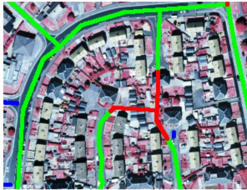
Figure 5.16. False extractions in Grangemouth subset 2 if context objects are not used. Correctly extracted roads in green, incorrectly extracted roads in red, missed extractions in blue.
