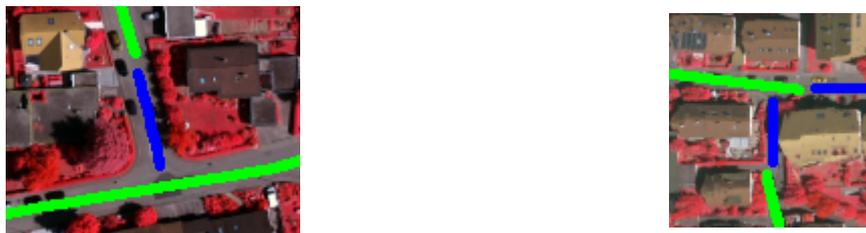
a. Missed connection due to small search radius. b. Missed connection due to geometric inaccuracy.
