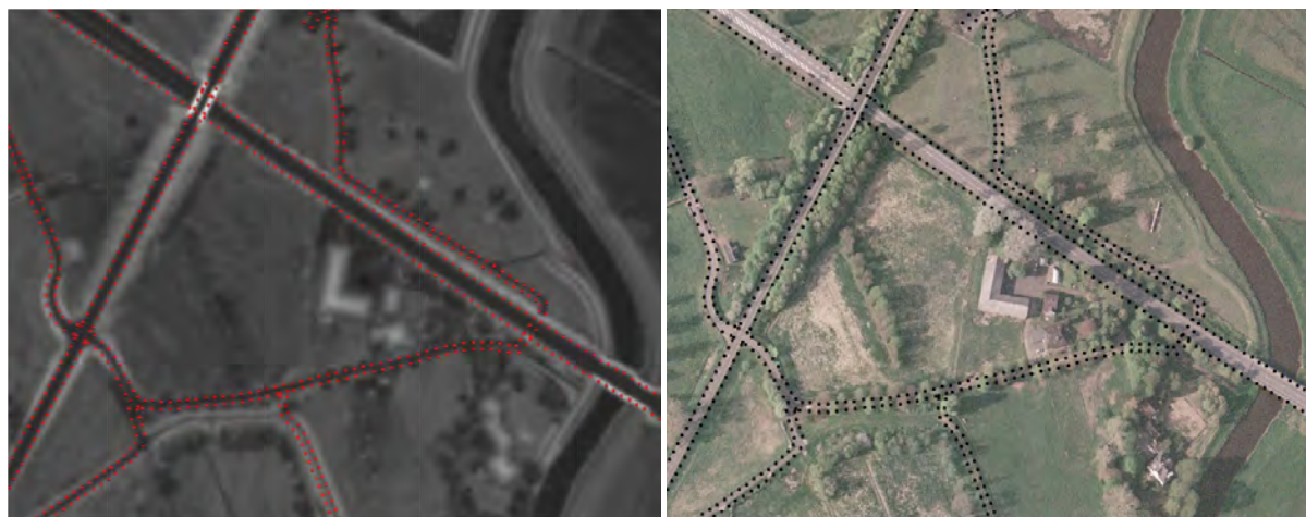
Figure 33. Detail of test site 1b: final ribbon snake (red and black dots); background: image energy from ALS (left); orthophoto (right).
