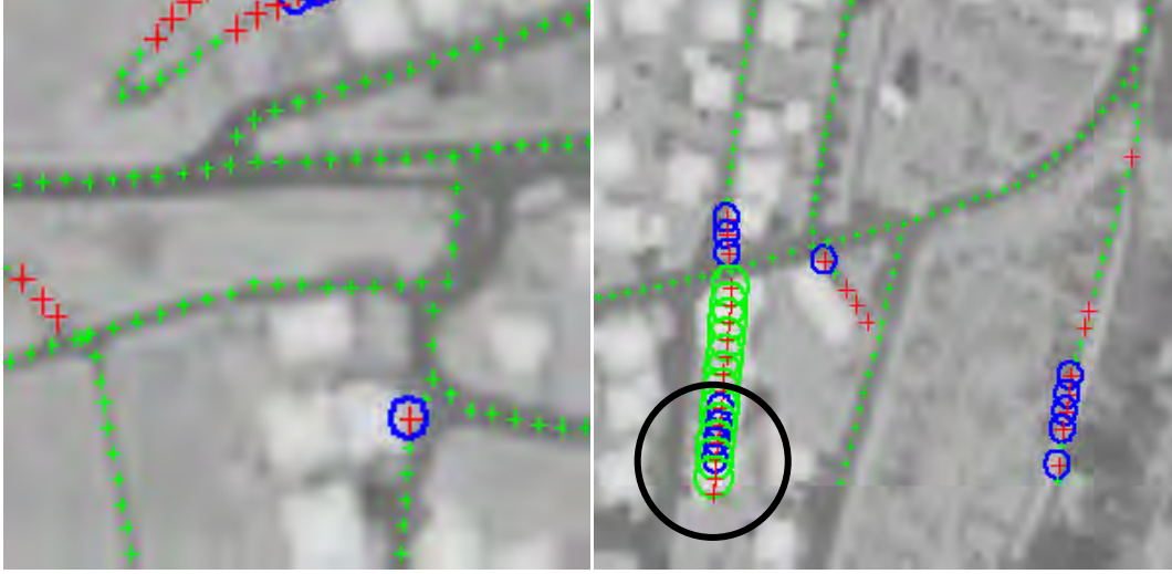
Figure 17. Detection of wrong contour parts in the two road networks of Fig. 16; crosses: image energy lower (green) or higher (red) than the mean value of all nodes, green circles: result of the first detector; blue circles: result of the second detector.
