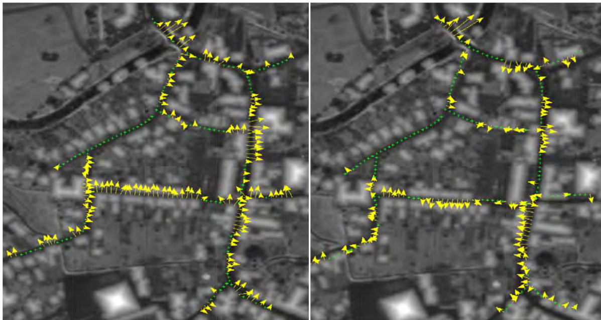
Figure 21: Distribution of the gradients of the image energy after 100 iterations: left: shifted initialisation (5 m; 5 m); right: rotated initialisation (0.05 rad) (background: image energy)
