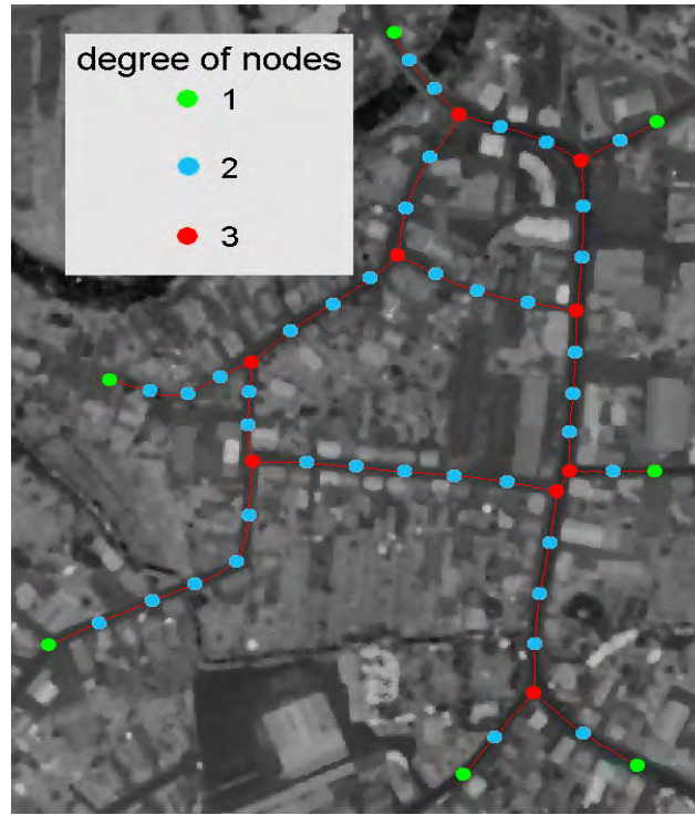
Figure 9. Topology of a road network represented by its centre lines. The degree of the nodes is indicated by the node colour (background: DSM+ALS intensity).
