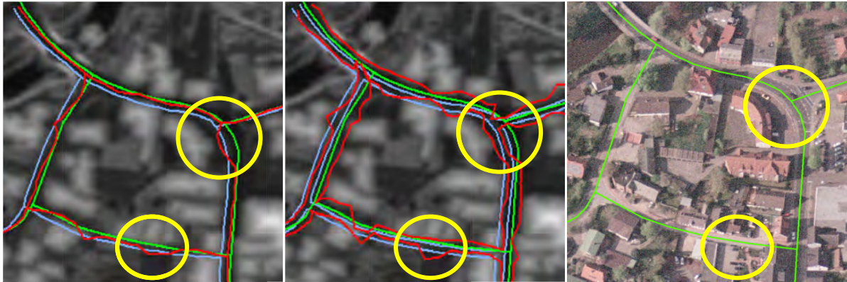
Figure 26. Optimisation results for the standard (left) and the ribbon model (centre) using very small weights for the internal energy ( \alpha = \beta = 0.01 ) (left and centre: background: image energy; blue: initialisation; red: final position; green: reference centre line, yellow circles: large errors) (right: background: orthophoto; green: reference centre line)
