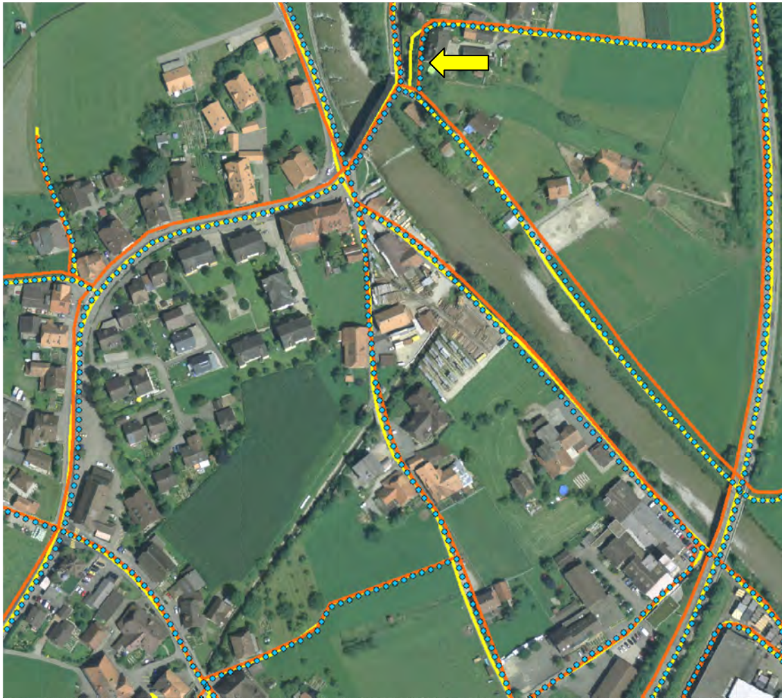
Figure 36. Part of test site 3a (data set Emmental, urban): centre line of ribbon snake model superimposed to an orthophoto. red: original vector data; yellow: reference; blue points: optimised snake nodes, yellow arrow: largest error.
