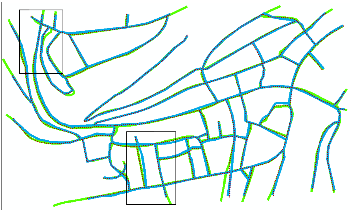
Figure 39. Test site 4 (data set Vaihingen, urban and rural): green: reference centre line; blue: initialisation; red dots: optimised snake nodes (central nodes of the ribbon); black rectangles: details in Figs. 40 and 41
