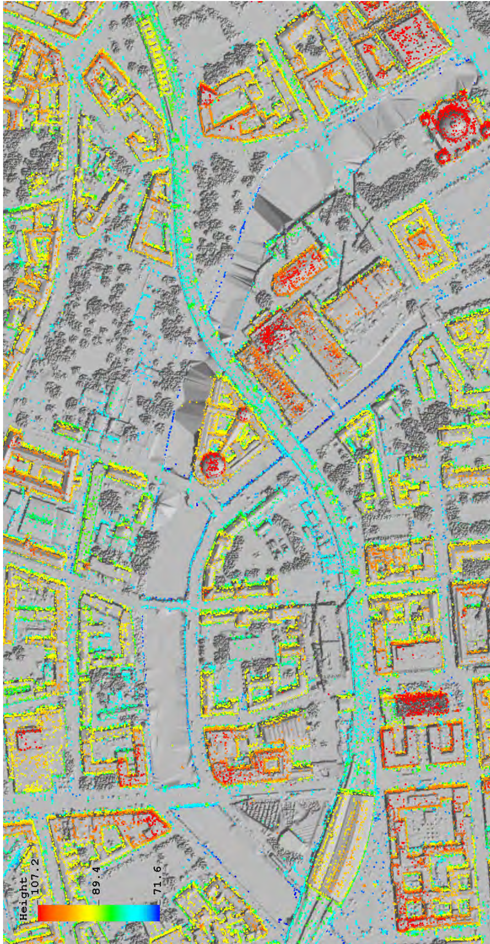
Figure 75: Top view on PS point cloud generated from fusion of 5 stacks of Berlin test site. In addition, a DSM of the area is included in the background. PS are color-coded by their height between approximately 72 m and 107 m. Visually, the fused PS point clouds already fit the reference surface (DSM) quite well. Hence, absolute positions could be estimated successfully.
