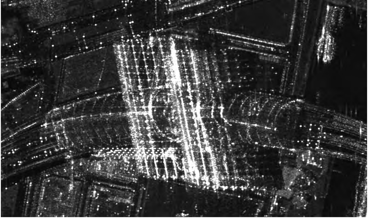
Figure 53. SAR image of central train station. The main parts can easily be identified: The two main building parts across the rail tracks, the two halls covering the tracks (to the left and right) and the tower, partly overlaid by one of the main building parts to the left. Azimuth: bottom-up, range: left-right.
