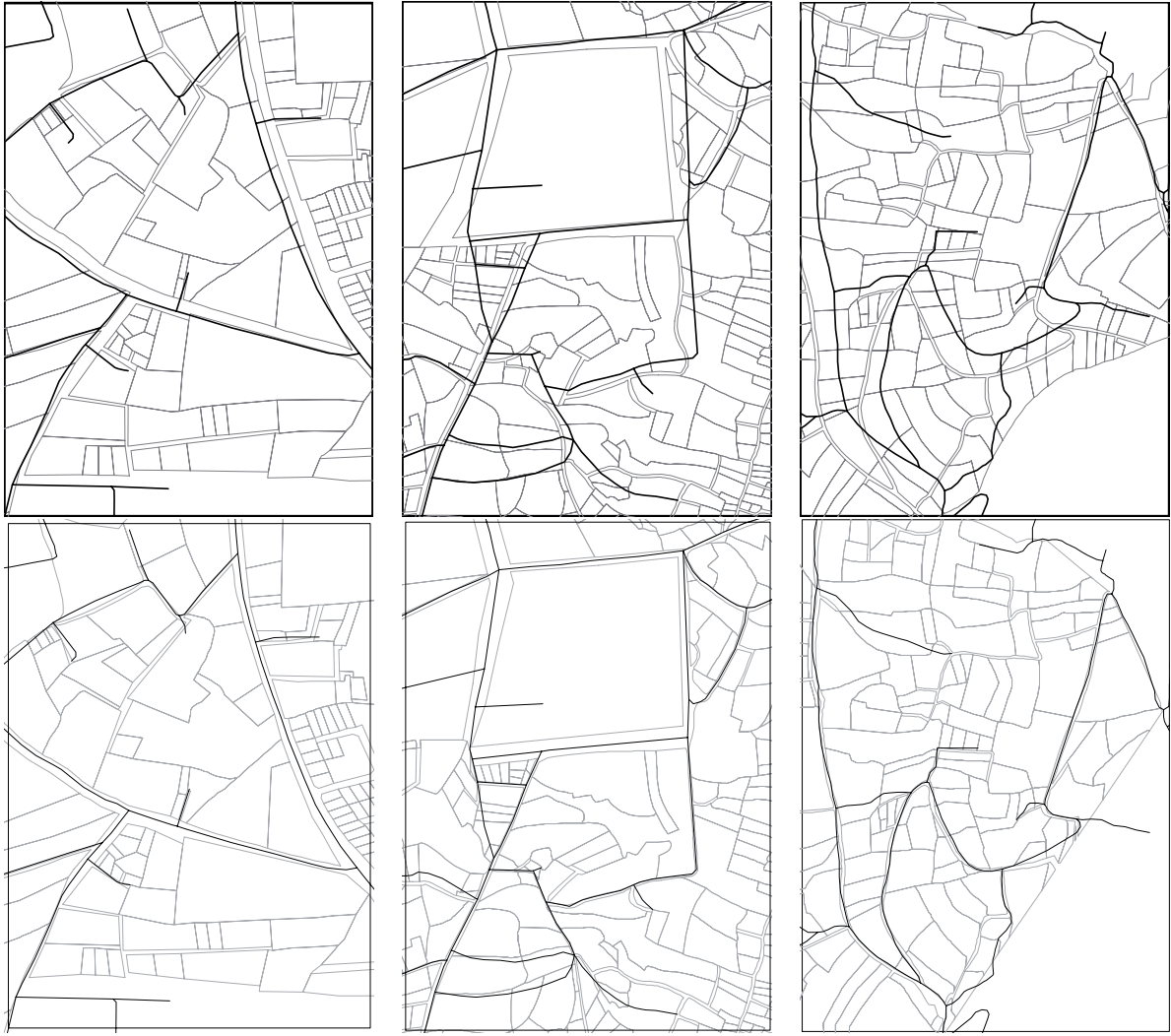
Fig. 6.16: Superposition of the cadastral (subject) dataset represented by parcels (light grey) and the topographical dataset represented by road network (black) showing extracts from the experimental data. The left, middle and right respectively represent 1, 2 and 3 boxes in Figure 6.15, while the top and bottom parts illustrate the situation before and after transformation respectively
