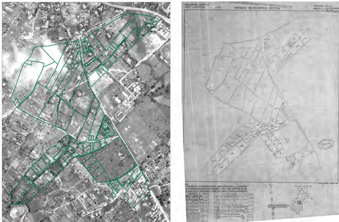
Fig. 3.4: Left -marking of parcel boundaries on un-rectified, uncontrolled and mosaicked aerial photographs, Right -resulting PID after tracing from the marked photographs
