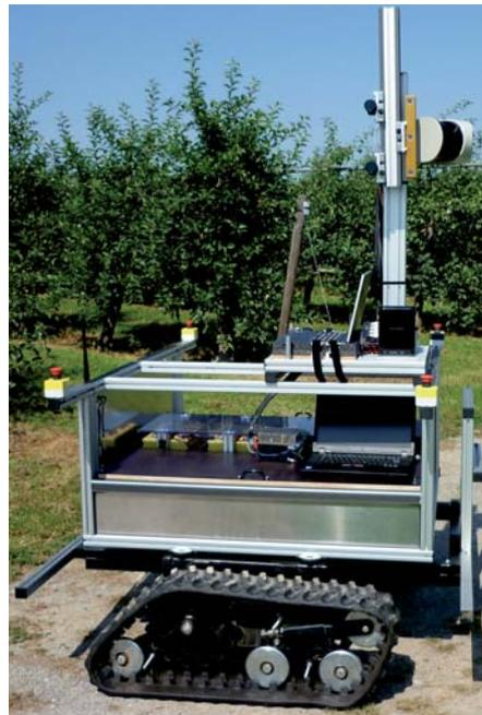
(b) University Of Hohenheim Unmanned Ground Vehicle (UGV) With ZHAW Measurement Pillar.
