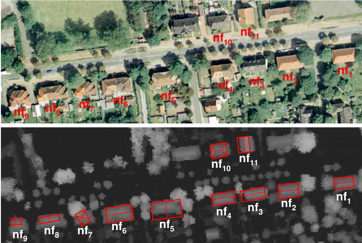
Figure 5.9: Results of non-flat-roofed building extraction: optical image with labelled buildings (top), and LIDAR DSM overlaid with final building footprints and marked ridge orientation (bottom)
