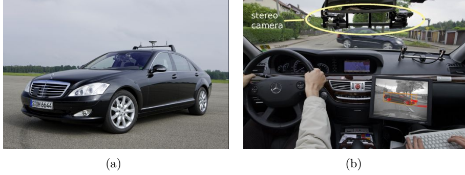
Figure 4.17.: (b) Mercedes-Benz demonstrator car used for testing of the proposed methods. (b) The stereo-system is mounted behind the windshield.
