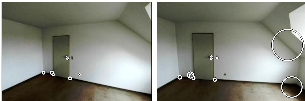
FIGURE 1.1: A pair of overlapping images showing a scene with sparsely textured surfaces, overlaid with a typical set of local features (Lowe, 2004). The number of features is critically low for applications like image orientation.
