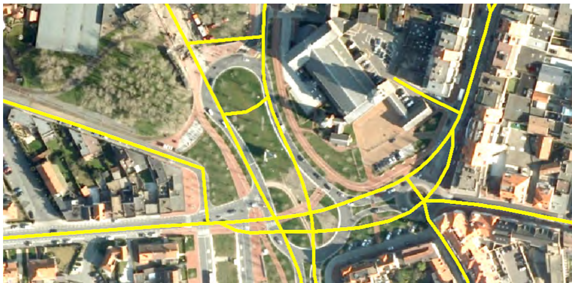
Figure 1.1.: Up-to-date imagery superimposed by an outdated road database.
