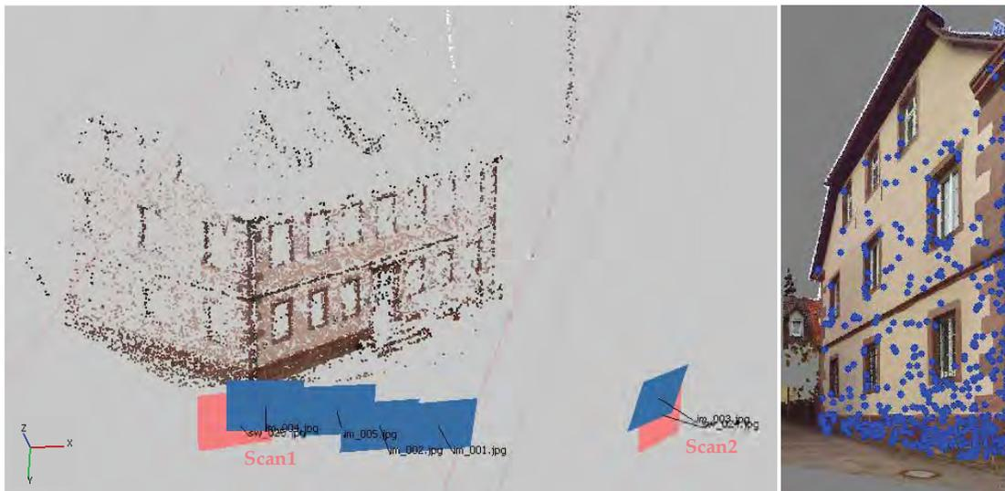
**Fig.7.21.** SfM output: sparse point clouds (colored), 5 camera positions (blue image planes) and 2 scan stations (pink image planes) of the Building 1 at the Hirsau Abbey dataset, aligned in one local coordinate system (left). 3D correspondences (478 keypoints) between the sparse point clouds and the laser data (of Scan1) which are used for the calculation of the seven- parameters, depicted on the corresponding RGB image (right).
