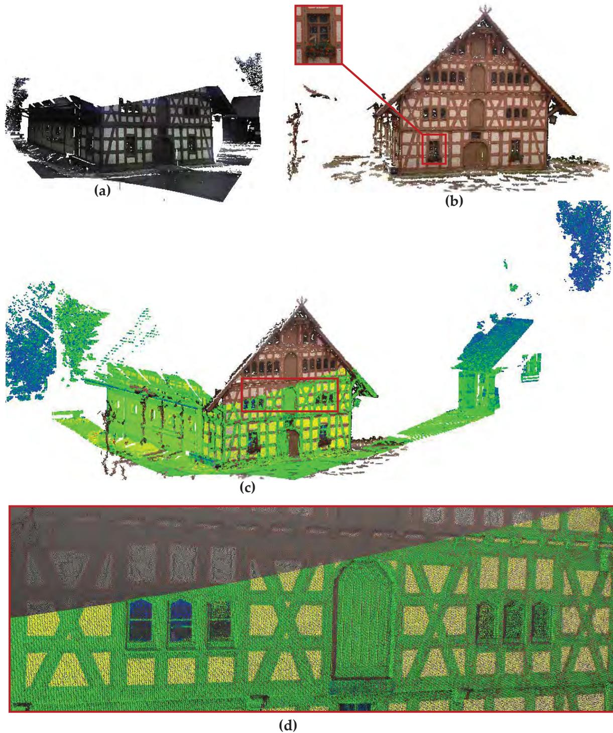
**Fig.4.9.** Dense image matching results using patch-based multi-view stereo (PMVS) algorithm. (a) 3D laser scanner point clouds, from one scan station, of the old farm house acquired by the Leica ScanStation HDS3000. (b) Dense image point clouds generated by the PMVS using the orthogonal iteration (OI) algorithm outputs, about 0.5 million pts. (c) Combined point clouds from (a), which is depicted with scalar fields & (b). (d) A close-up view for a window area depicted in (c).
