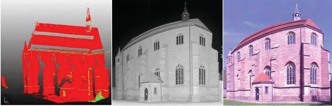
**Fig.3.2.** The Lady Chapel dataset, from the left, 3D laser scanner point clouds acquired by the Faro® Laser Scanner Focus<sup>3D</sup> at an approximate sampling distance of about 7 mm@10m distance, delivered Reflectance and RGB images.
