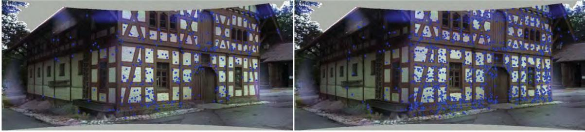
*Fig. 4.18. 3D-to-3D filtered correspondences (383 keypoints) between sparse point clouds and a laser scan of the old farm house dataset using only the features appeared in the corresponding RGB image (left). 3D-to-3D filtered correspondences (1064 keypoints) between sparse point clouds and a laser scan of the old farm house dataset using all projected sparse point clouds onto the corresponding RGB image (right).*
