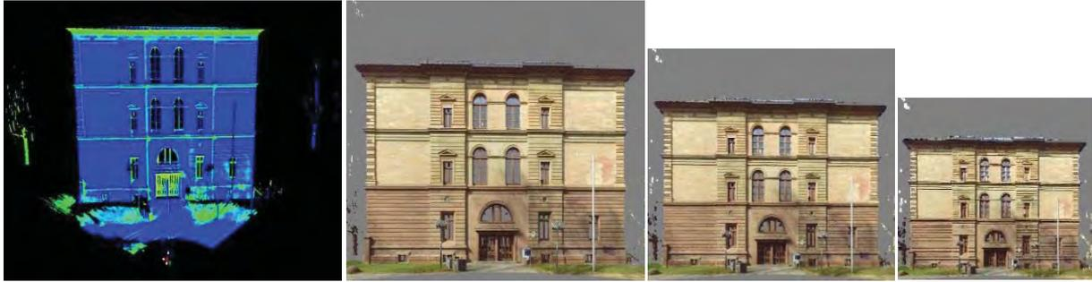
**Fig.3.6.** Dataset of Stuttgart University building, from the left, 3D laser scanner point cloud acquired by the Faro® Laser Scanner Focus<sup>3D</sup> and generated RGB images with different pixel footprints; interval distance in object space (2, 5 and 9cm).
