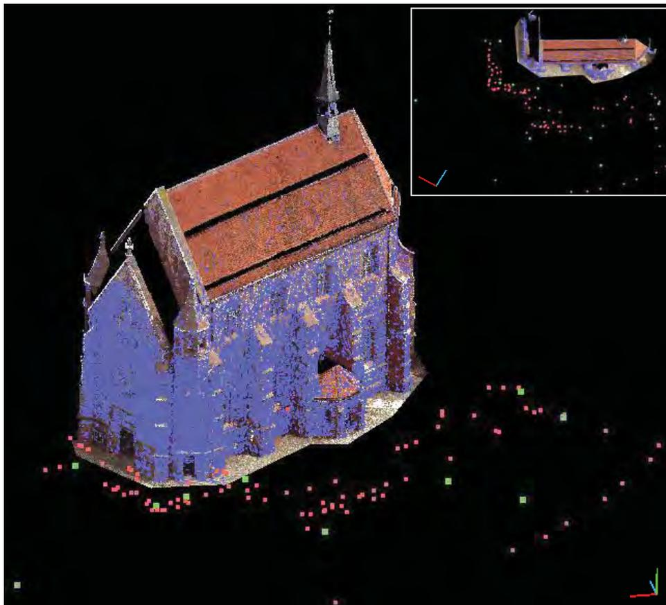
*Fig. 7.5. SfM output: sparse point clouds (blue), 97 camera positions (red dots), 10 scan stations (green dots) aligned in one coordinate system with laser point clouds from all 10 scan stations of the Lady Chapel dataset (colored). In addition, an ortho view of the former mentioned laser and sparse point clouds, camera positions and laser scanner stations and point clouds (upper right corner).*
