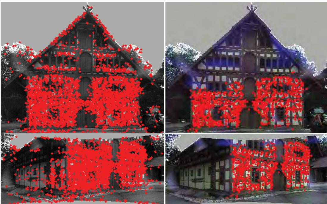
**Fig.5.8.** Old farm house dataset, removal of false correspondences. Correspondences (red dots), between a scan pair depicted on the corresponding generated RGB images, matched by the *kd-tree* descriptor comparison procedure with 4124 keypoints (left) and then filtered by RANSAC based on a closed-form space resection to obtain 1384 keypoints (right).
