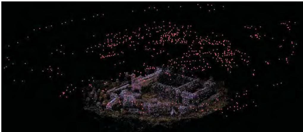
**Fig.6.3.** SfM output: sparse point clouds (colored points), 670 camera positions (red dots) of the Hirsau Abbey hand-made model.
