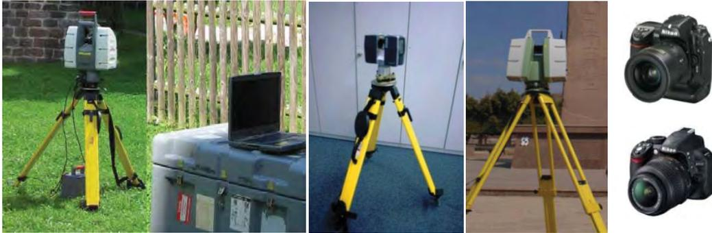
*Fig.7.3. The applied sensors, (From left to right) the Leica ScanStation HDS 3000, the Faro<sup>®</sup> Laser Scanner Focus<sup>3D</sup>, the Leica ScanStation C10, the NIKON D2X, 12 Mpx with 20 mm focal length (above) and the NIKON D3100, 14.2 Mpx with 24 mm focal length (bottom).*
