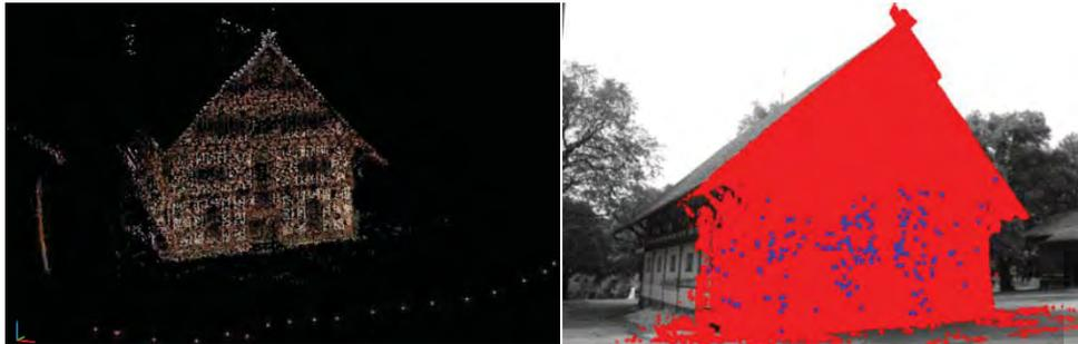
*Fig. 4.12. SfM output: sparse point clouds (colored), 19 camera positions (red dots) of the old farm house dataset (left). Reprojected dense image point clouds onto a camera image (red dots) and the resulted 3D correspondences (210 keypoints, blue dots) between the latter and the laser point clouds which are used for the calculation of the seven- parameters, depicted on the camera image (right).*
