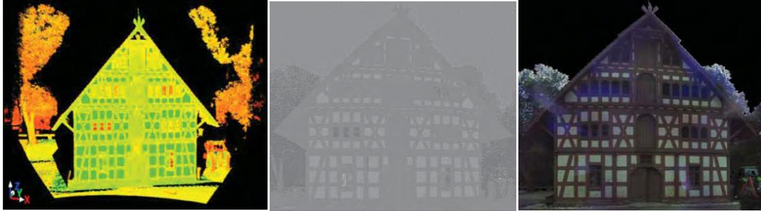
*Fig.3.1. The old farm house dataset, from the left, 3D laser scanner point cloud acquired by the Leica ScanStation HDS3000 at an approximate sampling distance of 2cm, generated Reflectance and RGB images using image matrix.*
