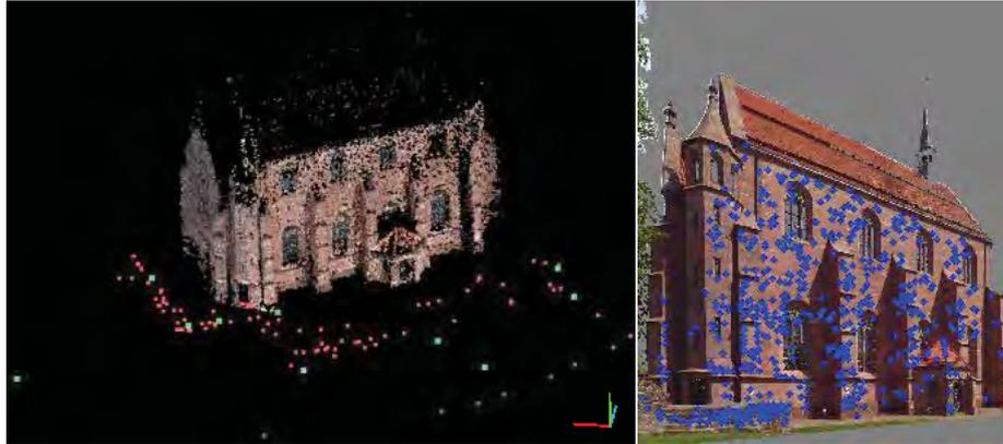
*Fig. 7.4. SfM output: sparse point clouds (colored), 97 camera positions (red dots) and 10 scan stations (green dots) of the Lady Chapel dataset, aligned in one local coordinate system (left). 3D-to-3D correspondences (415 keypoints) between the sparse point clouds and the laser data which are used for the calculation of the seven- parameters, depicted on the corresponding RGB image (right).*
