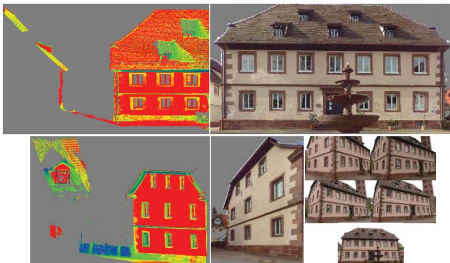
*Fig.7.20. The Building 1 at Hirsau Abbey dataset, from left to right, 3D laser scanner point clouds acquired by the Faro® Focus<sup>3D</sup> (at approximate point distance of about 7 mm @ 10 m distance) and the corresponding generated RGB image, for two non-overlapping scans; Scan1 above and Scan2 bottom. In addition, the used 5 camera images captured by the NIKON D2X (lower right corner).*
