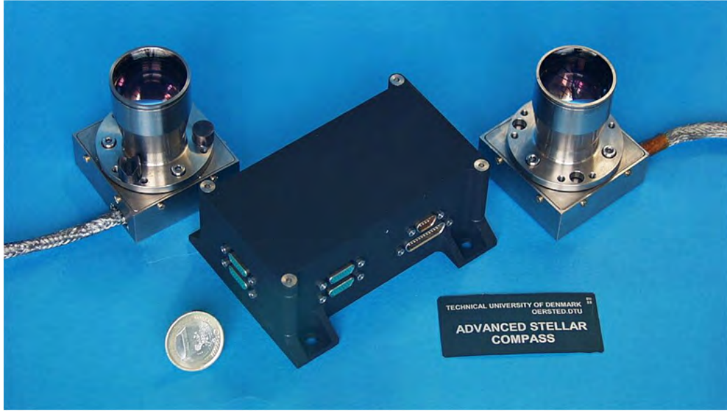
Figure 4.5: 2 CHUs and the DPU as manufactured at Technical University of Denmark.
