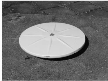
(b) Trimble Zephyr Geodetic
