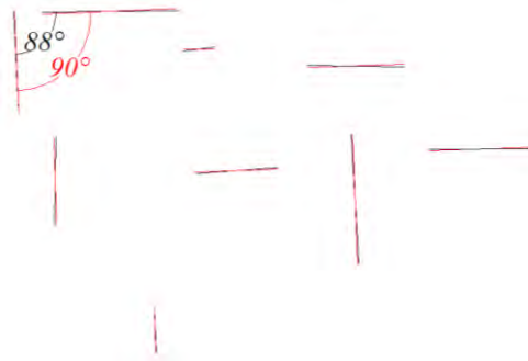
Figure 5.27: Regularization of boundary edges (on flat roof) extracted from images (black – before regularization, red – after regularization).
