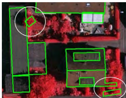
Figure 6.8: Erroneously extracted vegetation patches as roof planes and under-segmentation effect (Initial model results are overlaid on image data - white circle indicates the mentioned erroneous cases).
