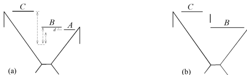
Figure 4.21: Outer-boundary simplification: (a) outer-boundary segments after regularization and (b) simplification. (Solid lines – outer- boundary segments, dash lines - the shortest distance between respective edge and segment centroid).
