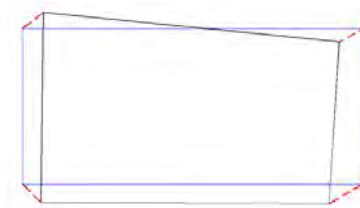
Figure 6.5: Difference of distance between vertices of reference and reconstructed polygon (blue – reference polygon, black – reconstructed polygon, red - displacement).
