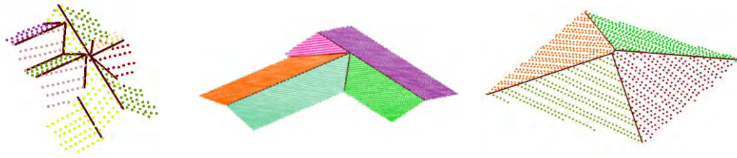
Figure 4.29: Geometrically fixed roof corners associated with ridge-lines.
