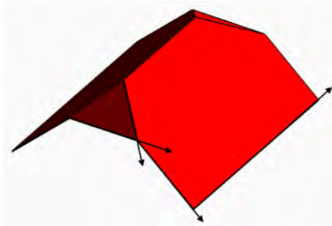
Figure 3.12: Geometric properties of the scene are re-defined again as constraints, (for a certain roof edge, it has a specific gradient which is helpful to discriminate the desired line among many omni-directional line segments in 3D).
