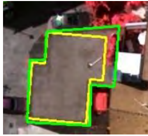
Figure 5.7: Ideal roof outlines which do not obey orthogonality or parallelism constraints (green – ideal edges extracted from image, yellow – reference line segments representing the edges of initial roof model).
