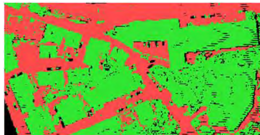
Figure 4.7: Classification results of a sample data set (red – terrain, green – off terrain segments, black – no data).
