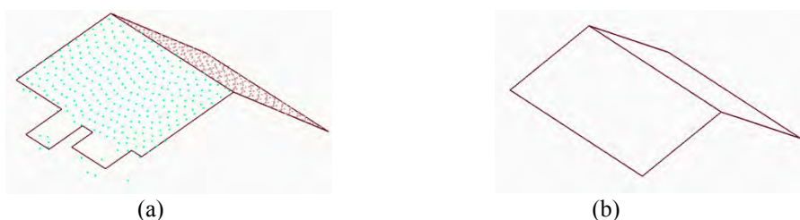
Figure 5.28: Defective contouring caused by under-segmentation: (a) erroneous overhangs due to merging of connected vegetation; and (b) after rectification the error.
