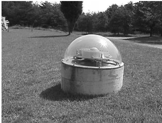
Figure 3.4: Typical IGS ground station (from [IGS 12a]).
