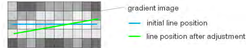
Figure 5.8: Local refinement of the matching between the image and model edge using gradient values
