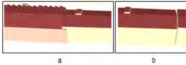
Figure 5.3: Examples of errors in snapping: a) small intrusions; b) gaps between the buildings. This error can be the result of inattentive modeling or numerical errors during translation between the formats.
