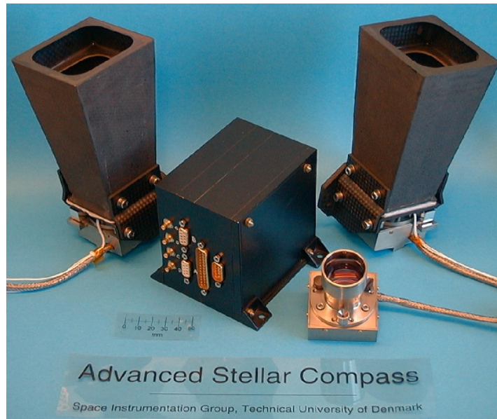
Figure 3.7: The star camera assembly consisting of the camera head units, baffles and the data processing unit as pictured by DTU. Note that onboard GRACE two (not three as shown here) star camera head units are mounted
