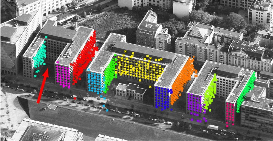
Figure 5.3: Result of the PS grouping approach. The color encodes the affiliation to individual facades. The projected PSs with the resulting grouping is shown. PSs which are not part of the regular pattern, i.e. irregular scatterers, are shown as crosses.
