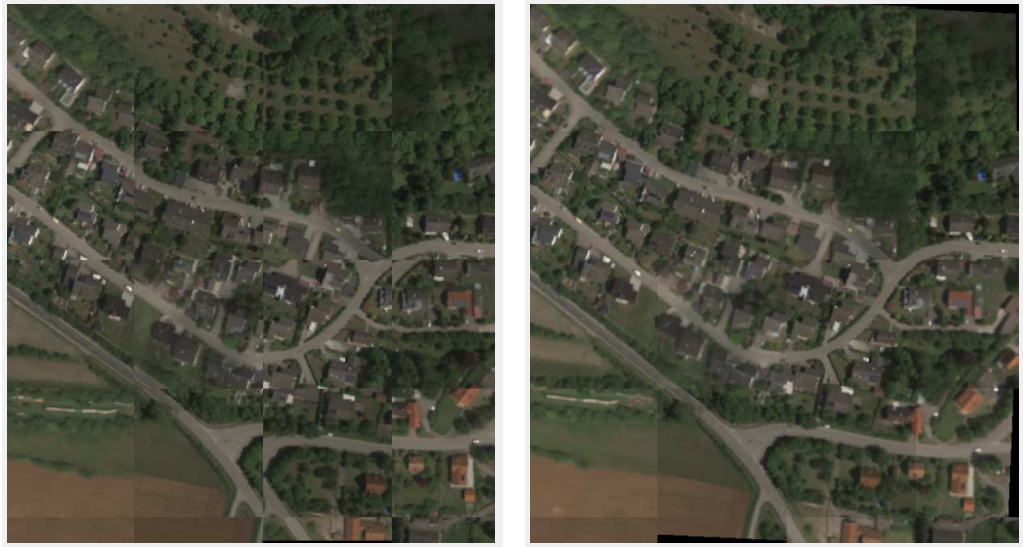
(a) Mosaic of georeferencing from raw GPS / INS data (b) Mosaic of georeferencing after GPS / INS post-processing, borsight correction and ECC maximization
