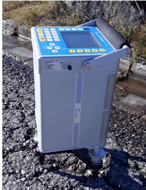
Figure 2.5: Scintrex CG-5 relative gravimeter in operation, leveled via tripod.
