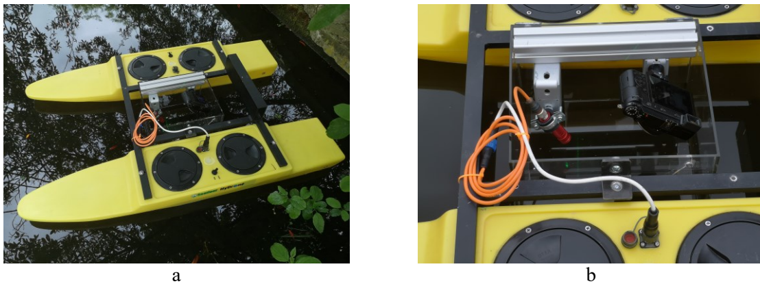
Fig. 3.4: Underwater laser triangulation sensor system integration in the UWV: set-up (a) and detail view (b).
