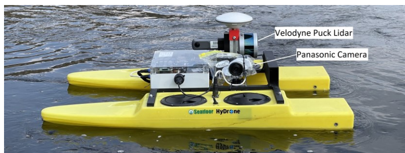
Figure 5: The uncrewed water vehicle used in this study. The Velodyne Puck lidar is attached vertically on the back, while the Panasonic camera is oriented towards the left in the direction of travel, protected with a soft plastic cover.
