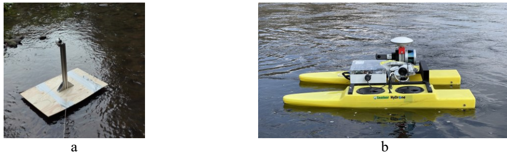
Fig. 2.1: Development stages of the UWV. From a towed wooden board on plastic bottles (a) to a remote controlled multi sensor platform (b).
