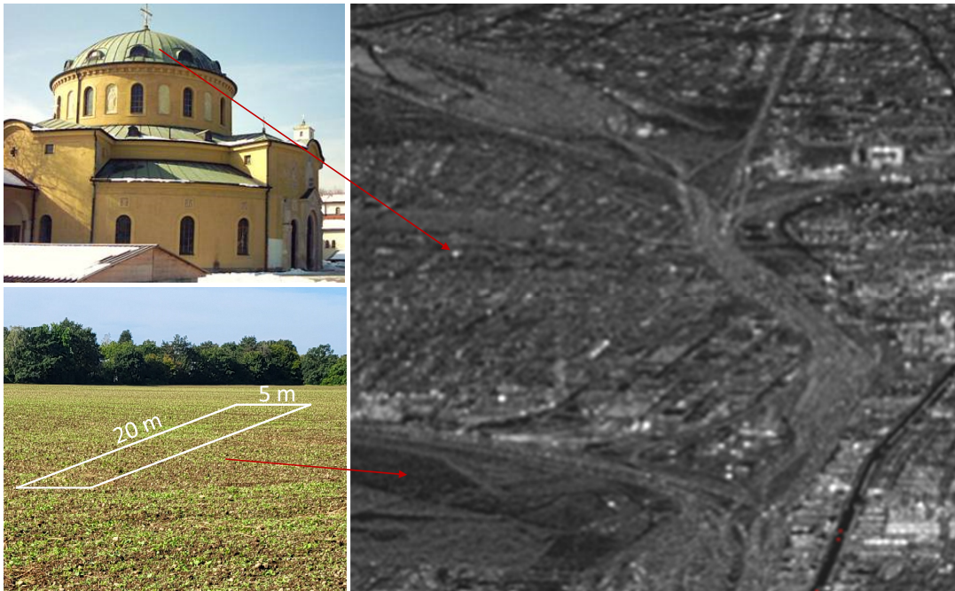
Figure 2.1: SAR scene amplitude (right image), point scatterer example (upper left image) and distributed scatterer example (lower left image).
