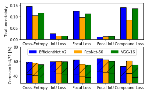
Figure 2. Total uncertainties and corrosion class related metrics of Deeplab V3+ models with respect to validation set consisting of different backbones and trained on various loss functions. The hatched bar sections indicate the difference between IoU and F1 score.
