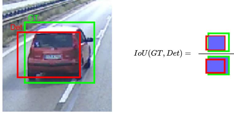
Figure 6.2: IoU for a 2D bounding box in image coordinates. Note, that these metric can also be applied to other types of shapes and volumes, like OBBs.
