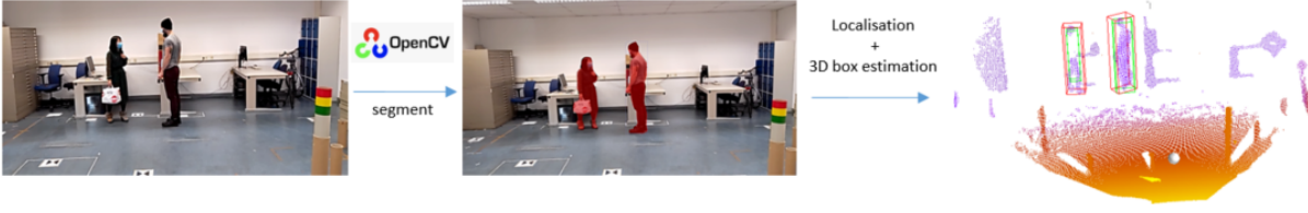
Figure 6.6: The pipeline implementation for MaskRCNN where raw RGB image, depth and the masks (in red) from the opencv segmentation are used to estimate the 3D bounding box for pedestrians in the scene.
