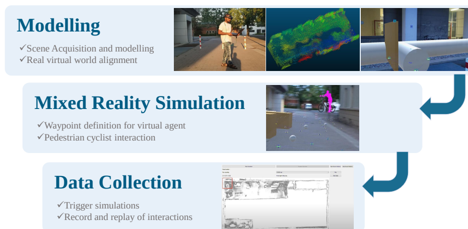
Figure 8.9: The workflow proposed framework that includes modeling- the creation of a test site, MR Simulation- interactions with virtual content and the data capture from the interaction experiment using the secondary interface.
