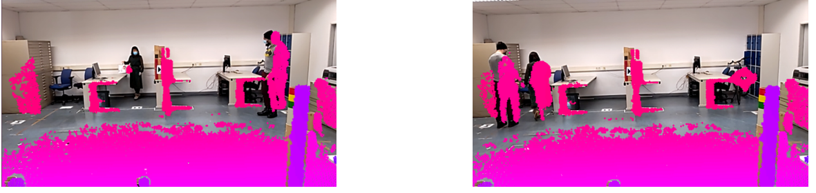
Figure 5.7: The Figure visually illustrates the errors in depth projection (highlighted with bright colours) using both the intrinsic and extrinsic parameters shared by Hololens research mode (Un-gureanu et al. 2020).
