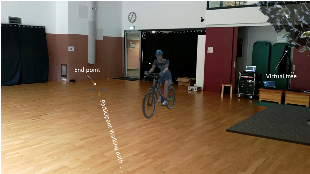
Figure 8.17: Mixed reality view of the crossing cyclist as seen from the Hololens. The figure shows the walking path along with the virtual tree that was added to the scene.
