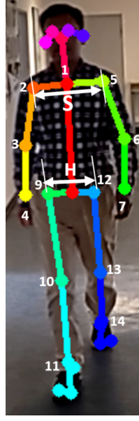
Figure 6.1: Openpose (Cao et al. 2017) based key-point detection with the dominant keypoints (S and H) that are considered for the Hand crafted features.
