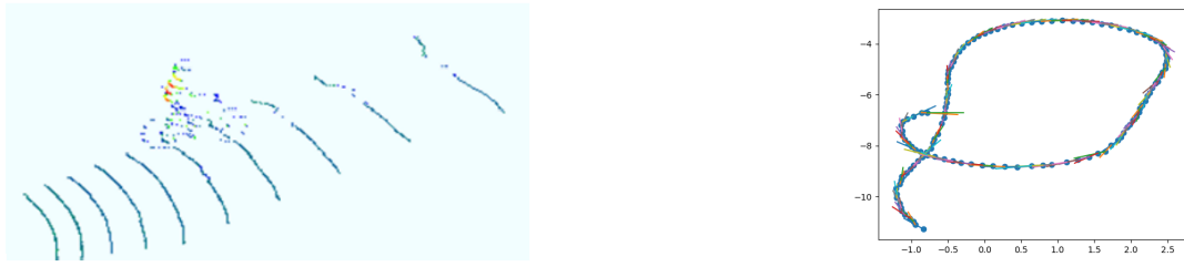
Figure 8.15: Figure on the left indicates the raw pointcloud (with the cyclist) captured using the 3D scanner and the right figure shows the extracted path and the rate of change of heading (indicated by tangential lines) for each time stamp.
