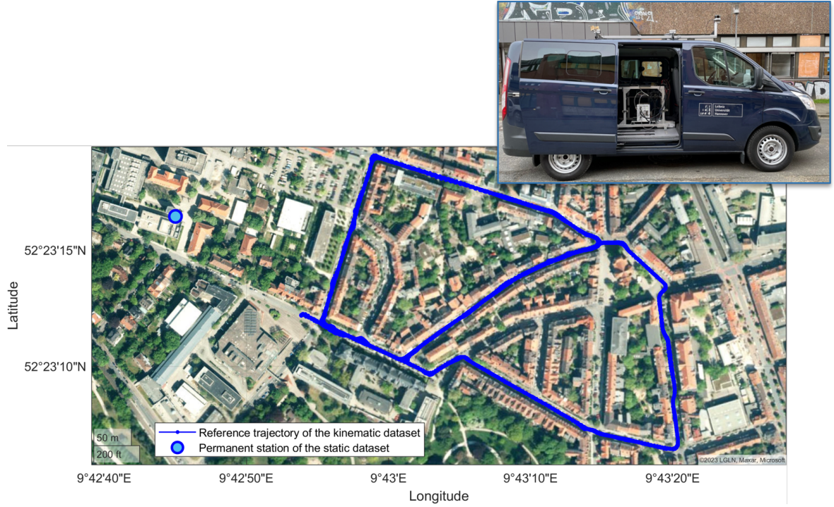
Figure 6.4: Data collection: the permanent station collecting the static dataset and the trajectory of the kinematic dataset are marked in the map as the light blue dot and dark blue lines, respectively.
