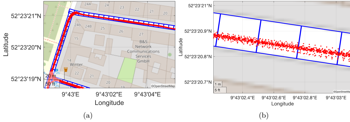
Figure 4.16: GNSS Feature Map box polygon assignment. (a) trajectory sample with generated boxes in blue and trajectory points in red, (b) zoom-in for depicting the large data pool.
