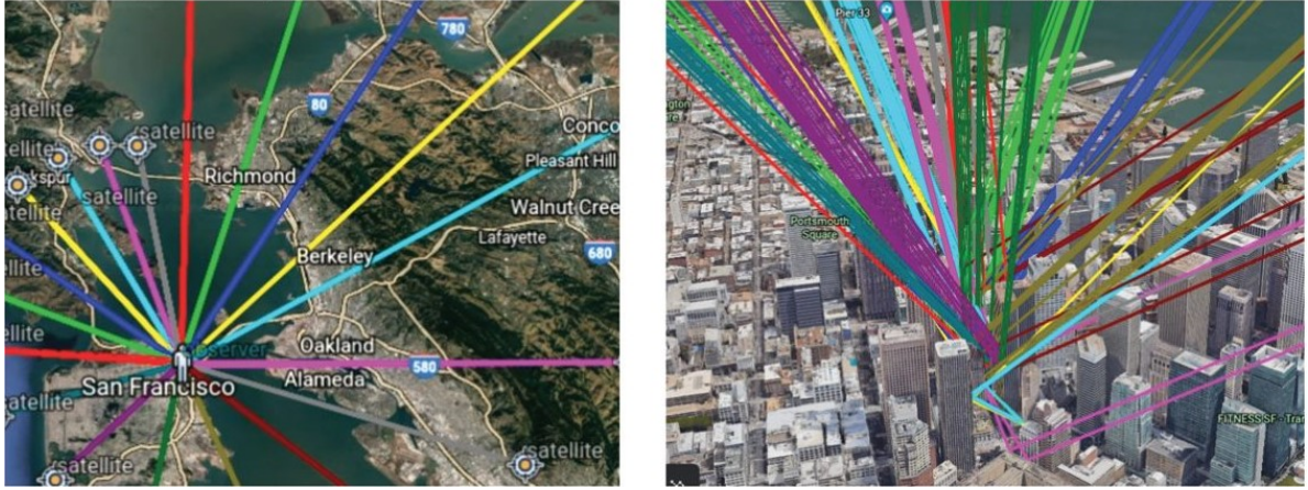
Figure 2.9: Exemplary situation of ray tracing for a given situation in San Francisco, USA. The right image is a zoom-in plot of the left image. Source: van Diggelen (2021).
