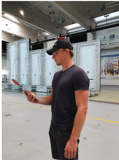
Figure 6.4: Tags placement on user UE and a cap worn by the user.
